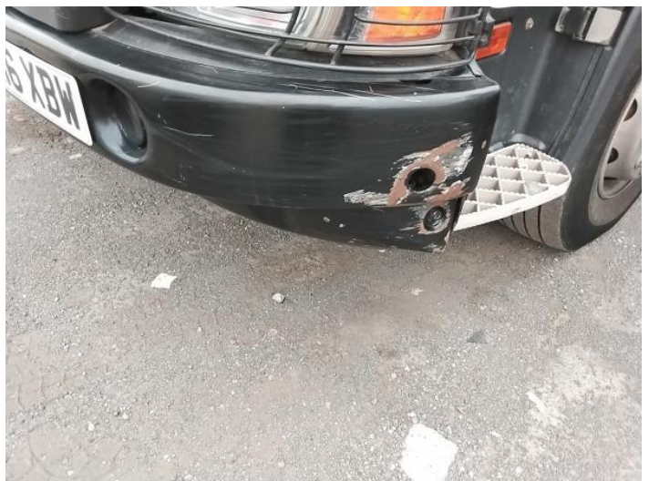
2: Bumper Front Dented With Paint Damage
