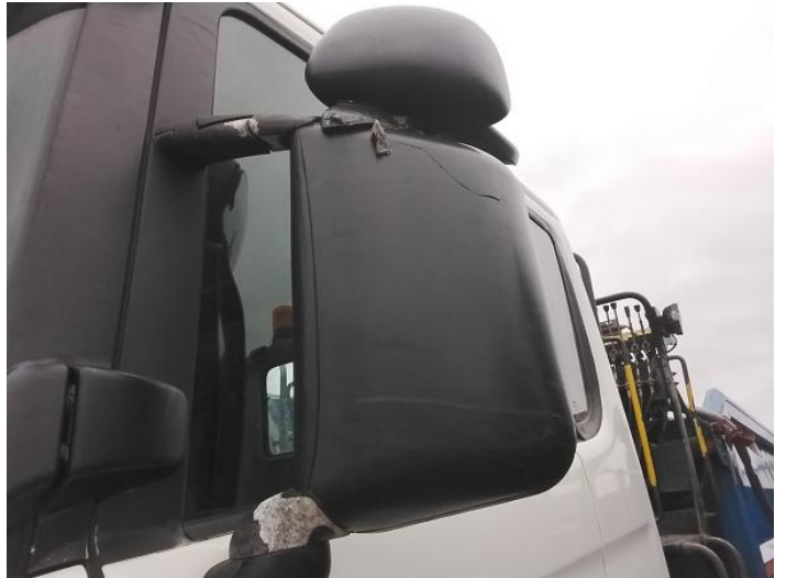
4: Door Mirror Assy nsf Broken Replace
