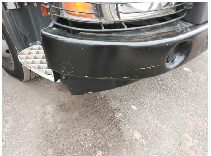
8: Bumper Front Scratched Over 100mm Thru Paint
