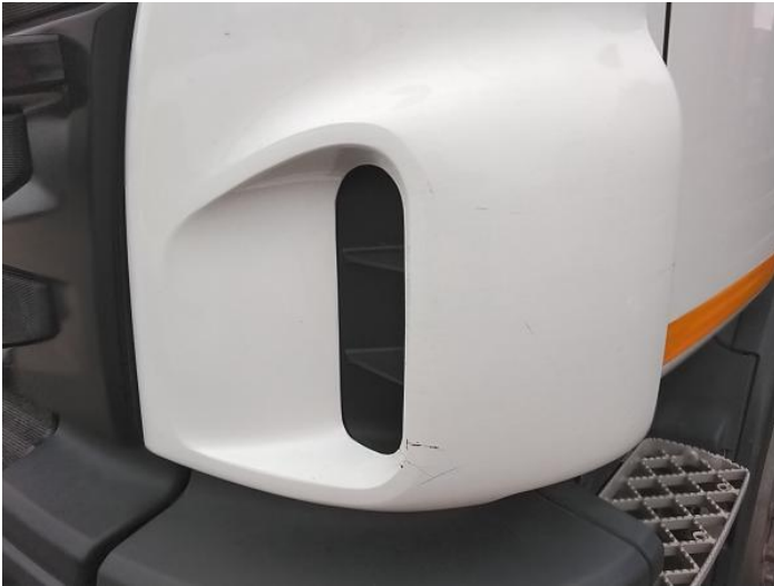
3: Panel Front Cracked Replace
