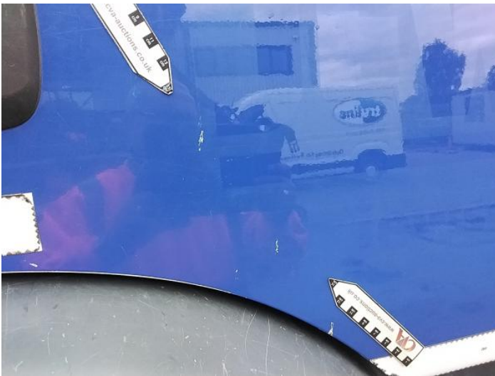
5: Door osf Dented With Paint Damage
