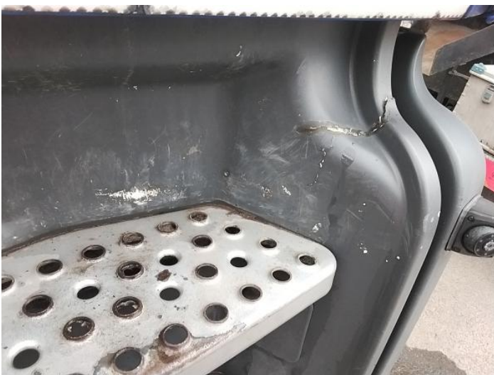
7: Wing osf Cracked Replace
