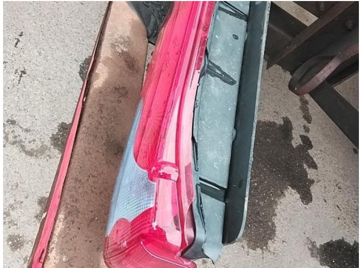
4: Lamp osr Broken Replace
