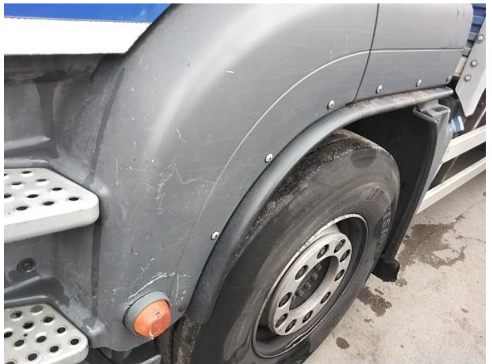
2: Wing nsf Scratched Over 25mm Thru Paint
