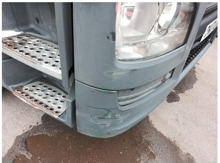
8: Bumper Front Scratched Over 100mm Thru Paint
