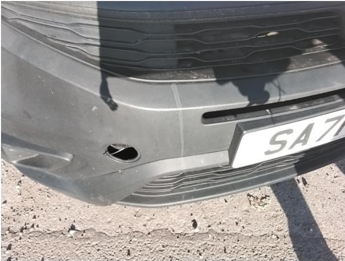
3: Bumper Front Moulding Missing Replace
