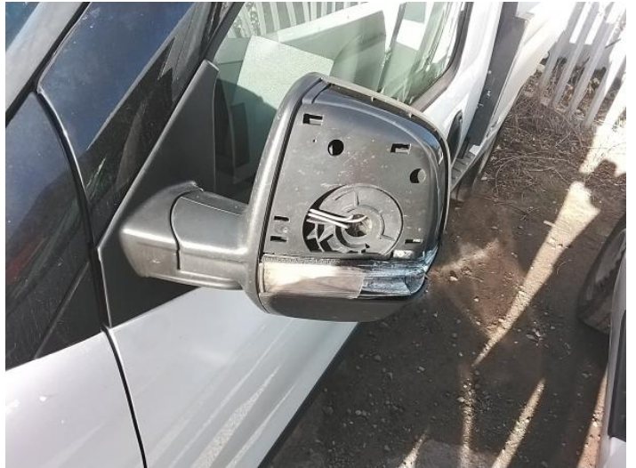
4: Door Mirror Assy nsf Broken Replace
