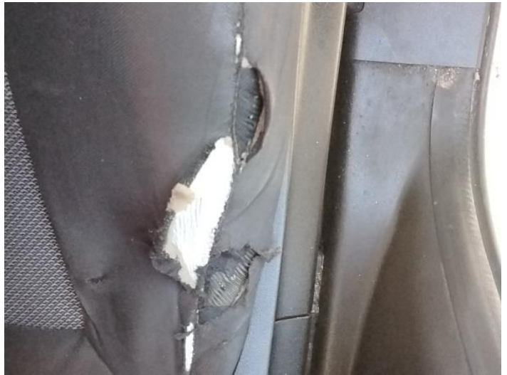
12: Seat Base Cover osf Torn Over 3mm
