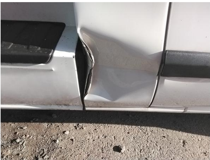
7: B Post os Cracked Replace
