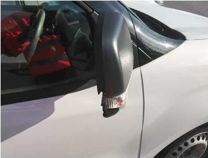
9: Door Mirror Assy osf Broken Replace
