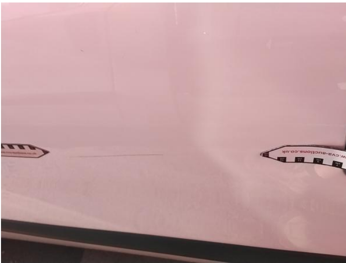
5: Door nsf Scratched Over 25mm Thru Paint
