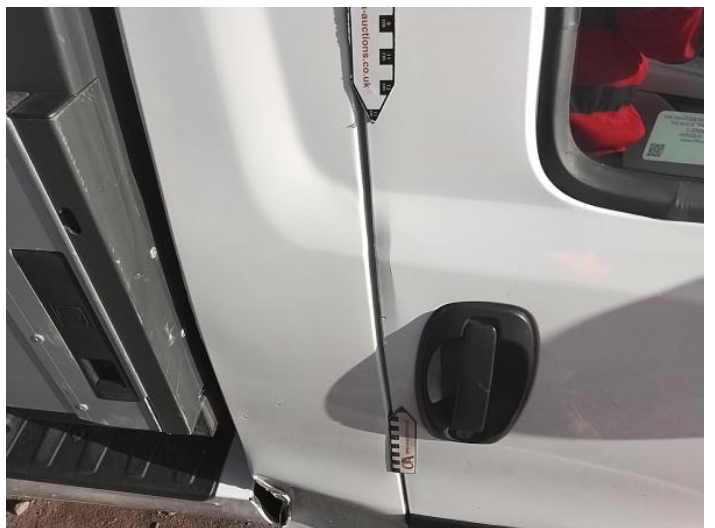
8: Door osf Dented With Paint Damage
