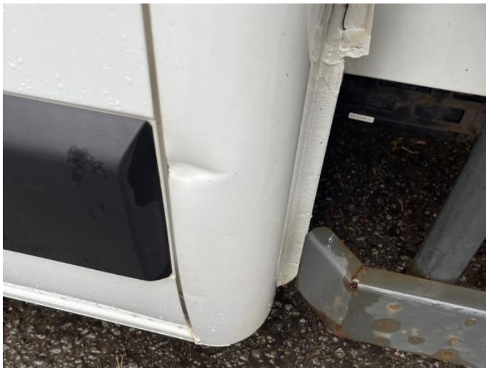
9: D Post ns Dented Over 30mm
