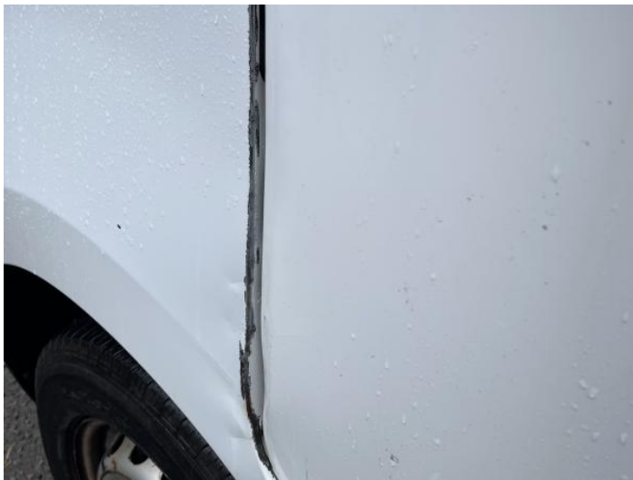
11: Door osf Dented With Paint Damage
