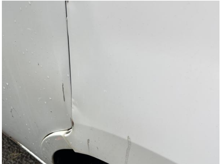
4: Wing osf Dented With Paint Damage
