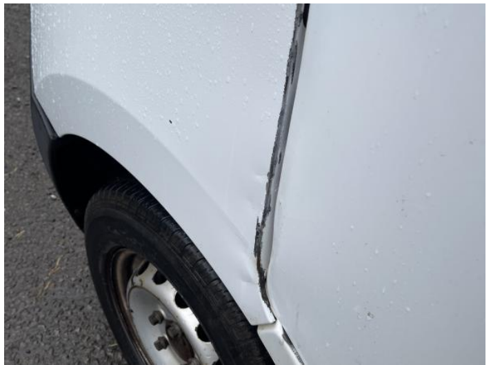
12: Wing nsf Dented With Paint Damage
