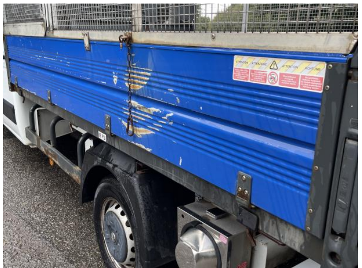
8: Qtr Panel nsr Dented With Paint Damage
