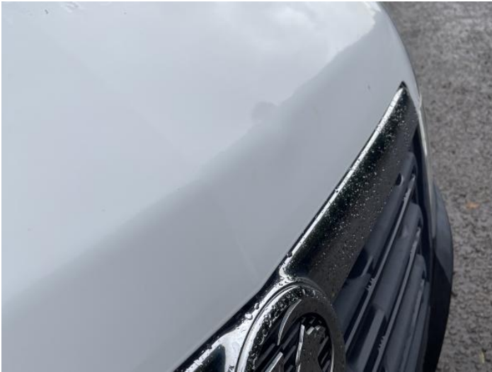
3: Bonnet Dented Over 30mm
