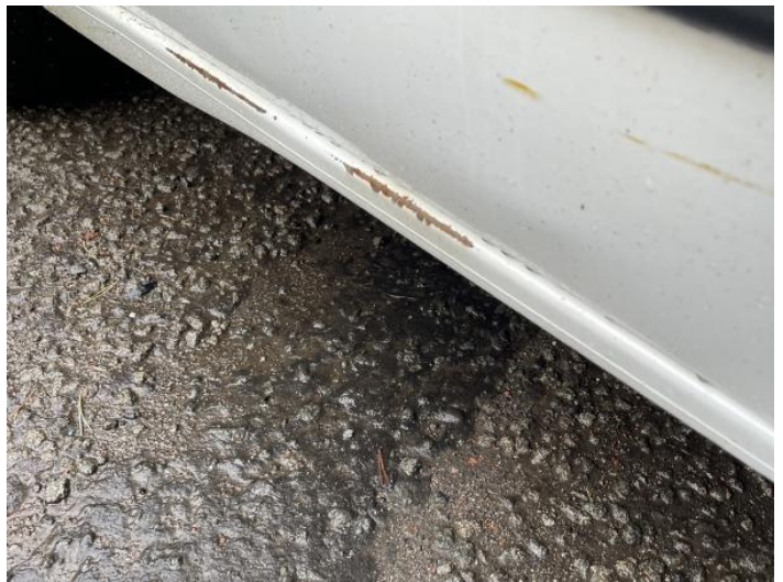
10: Sill ns Dented Over 30mm
