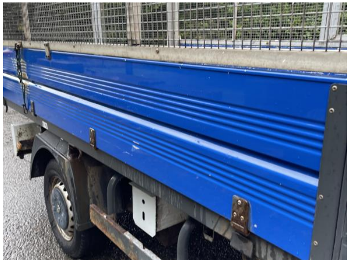
6: Qtr Panel osr Dented With Paint Damage
