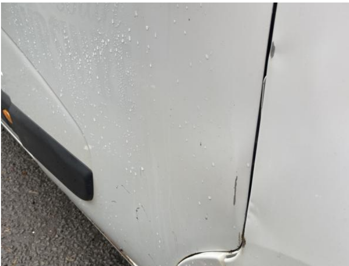
5: Door osf Dented With Paint Damage
