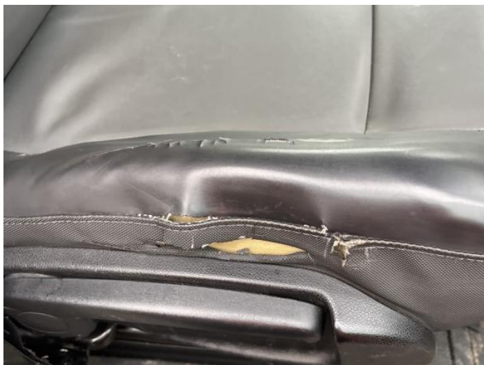
1: Seat Base Cover osf Torn Over 3mm
