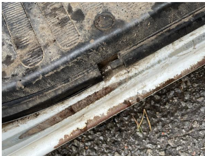
2: Sill os Rusted Over 5mm
