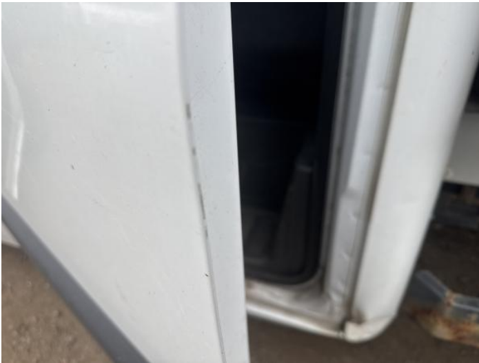
11: Door nsr Chipped Edge Chip
