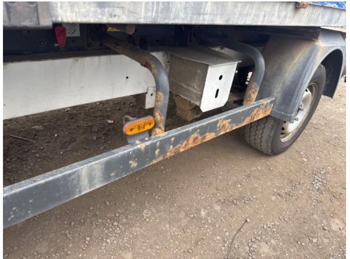
12: Qtr Panel nsr Rusted Over 5mm
