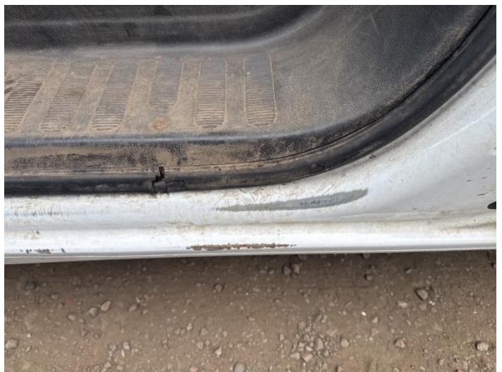
8: Sill ns Scratched Over 25mm Thru Paint
