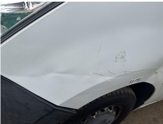
7: Wing nsf Dented With Paint Damage
