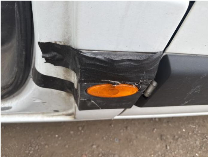
9: Qtr Panel Moulding ns Broken Replace
