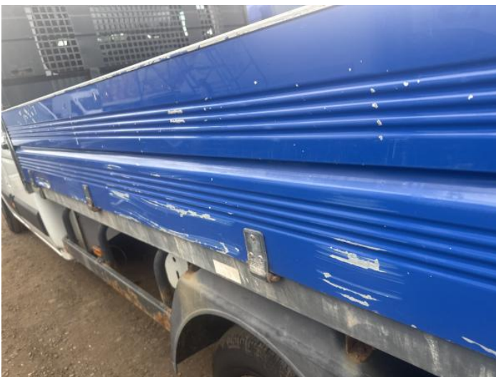
13: Qtr Panel nsr Scratched Over 25mm Thru Paint
