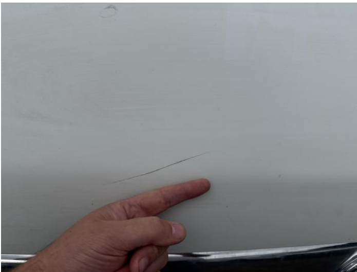
5: Bonnet Scratched Over 25mm Thru Paint
