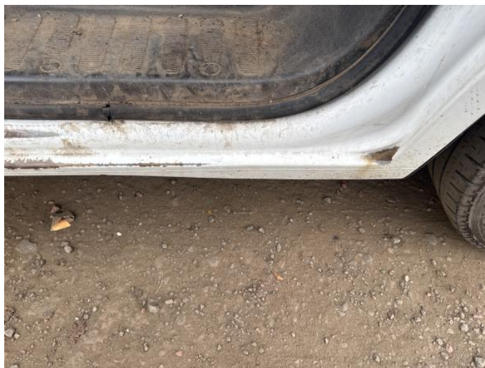
2: Sill os Rusted Over 5mm
