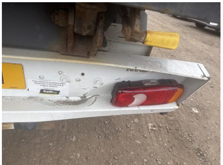
14: Bumper Rear Dented With Paint Damage
