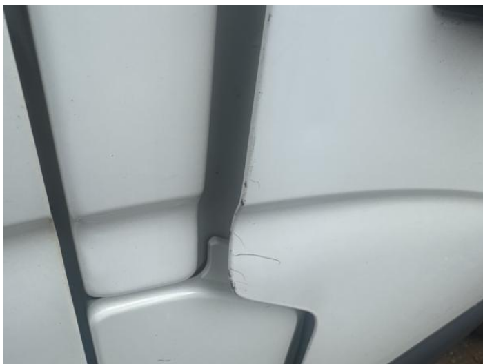
1: Door osf Chipped Edge Chip
