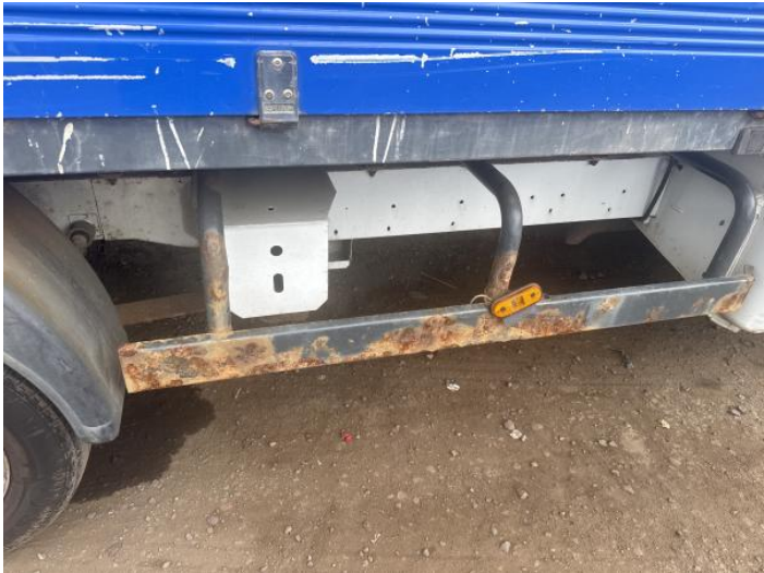
16: Qtr Panel osr Rusted Over 5mm
