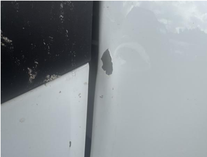
3: Wing osf Dented With Paint Damage
