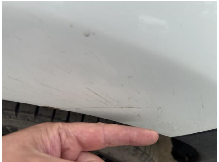
4: Wing osf Scratched Over 25mm Thru Paint
