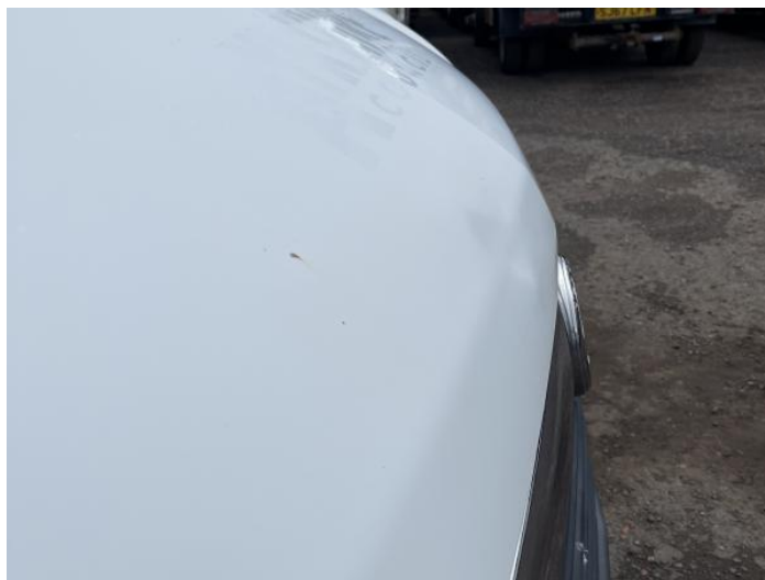
2: Bonnet Dented With Paint Damage
