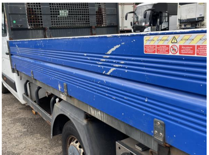
8: Qtr Panel nsr Dented Over 30mm
