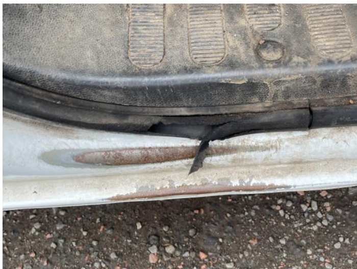
1: Sill os Rusted Over 5mm
