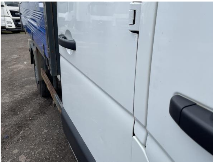
5: Door osr Dented Over 30mm
