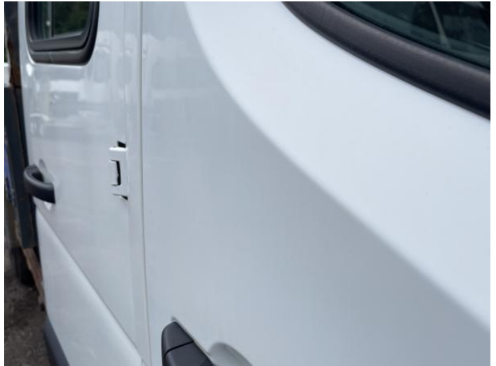
4: Door osf Dented Over 30mm
