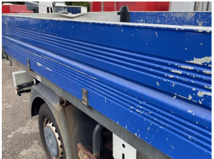
6: Qtr Panel osr Dented With Paint Damage
