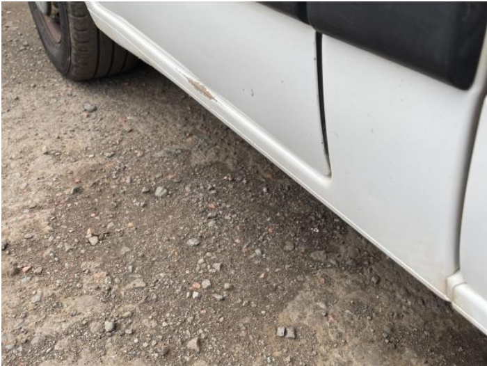
9: Sill ns Dented Over 30mm
