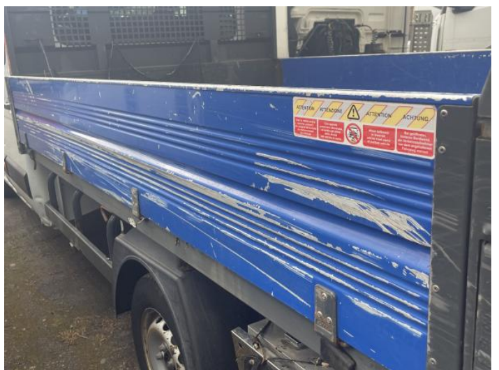
8: Qtr Panel nsr Dented With Paint Damage
