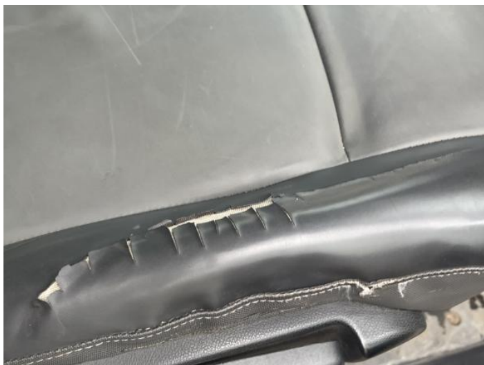
1: Seat Base Cover osf Torn Over 3mm
