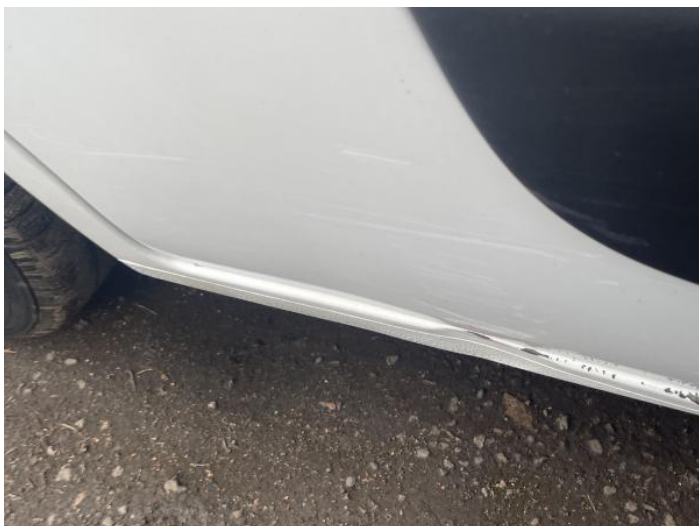
9: Door nsf Dented With Paint Damage
