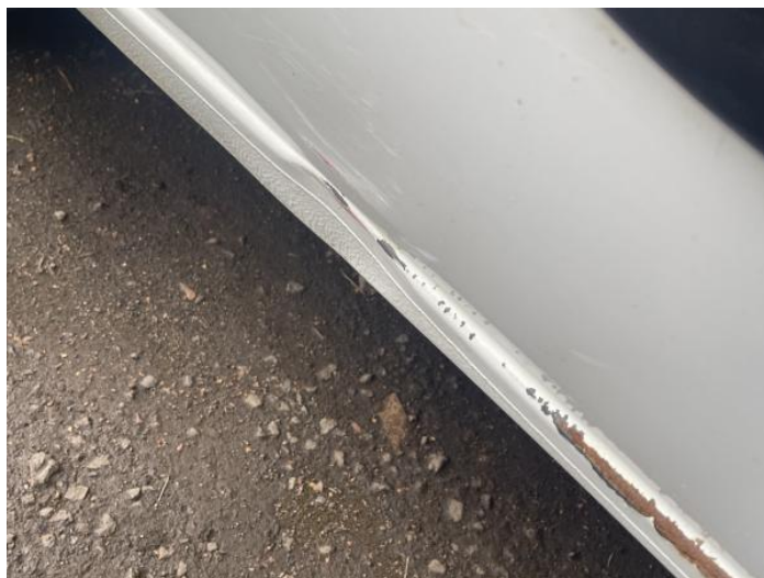
10: Sill ns Dented With Paint Damage
