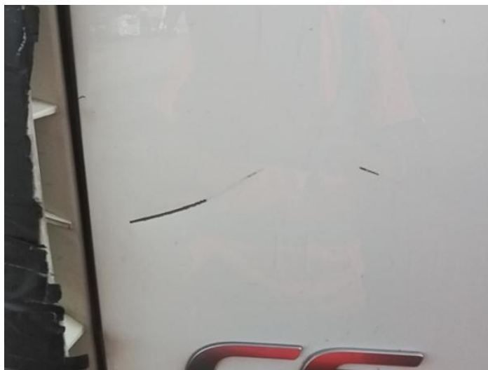
2: Door nsf Scratched Over 25mm Thru Paint
