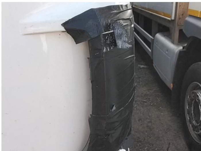
1: Panel Front Poor Previous Repair Poor Colour
