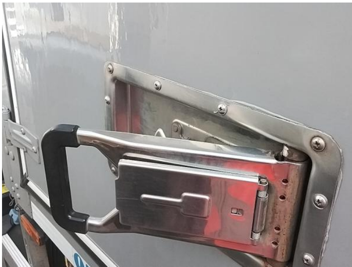
3: Handle Outer nsr Broken Replace
