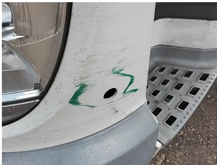
2: Bumper Front Scratched UpTo 25mm Not Thru Paint
