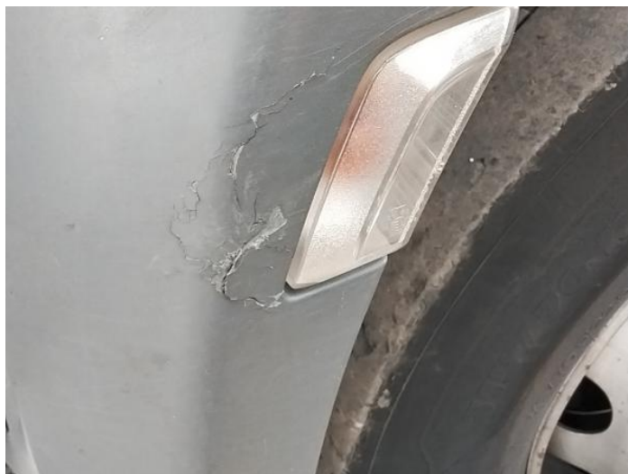
4: Wing nsf Cracked Replace
