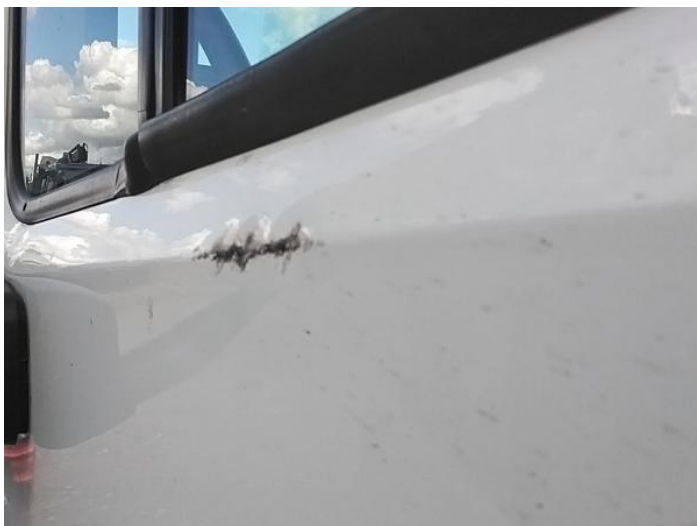
3: Door nsf Dented Hail - Severe
