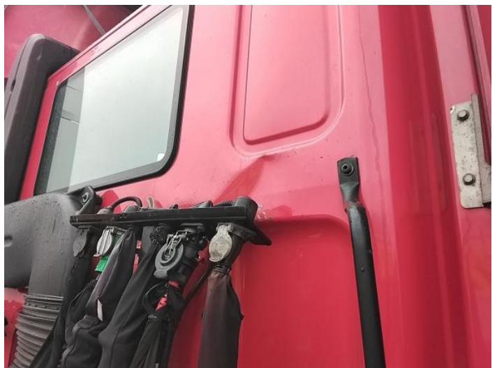
8: Panel Rear Dented With Paint Damage
