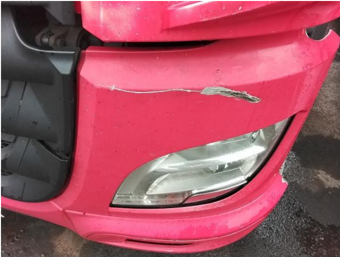
3: Panel Front Cracked Replace
