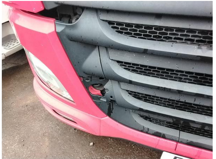
2: Bumper Front Moulding Missing Replace
