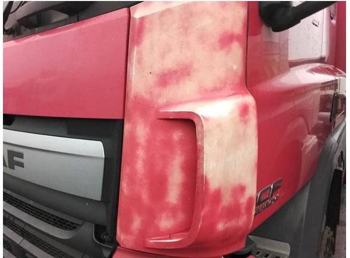
4: Panel Front Poor Previous Repair Poor Colour
