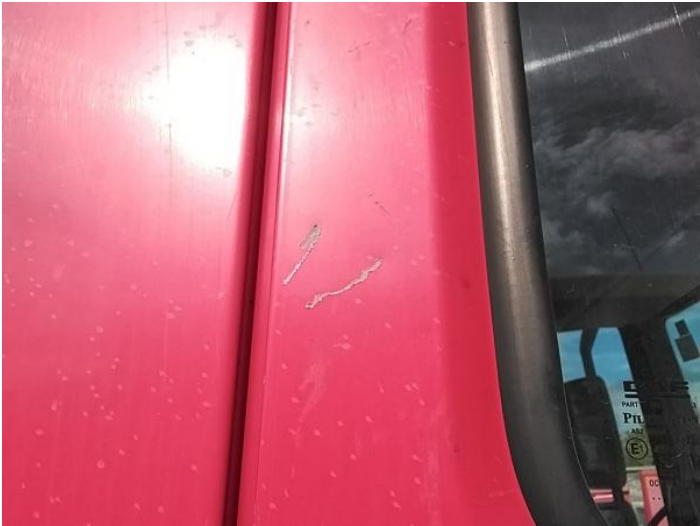
3: Door osf Scratched Over 25mm Thru Paint
