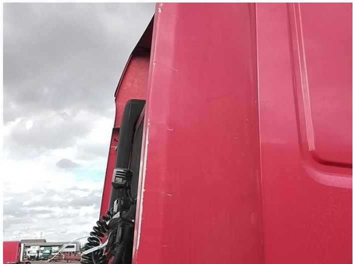
2: Tailgate Trim Panel Scuffed (Unpainted) Over 100mm
