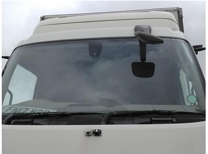
10: Screen Front Chipped UpTo 10mm
