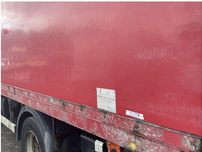
10: Qtr Panel nsr Rusted Over 5mm
