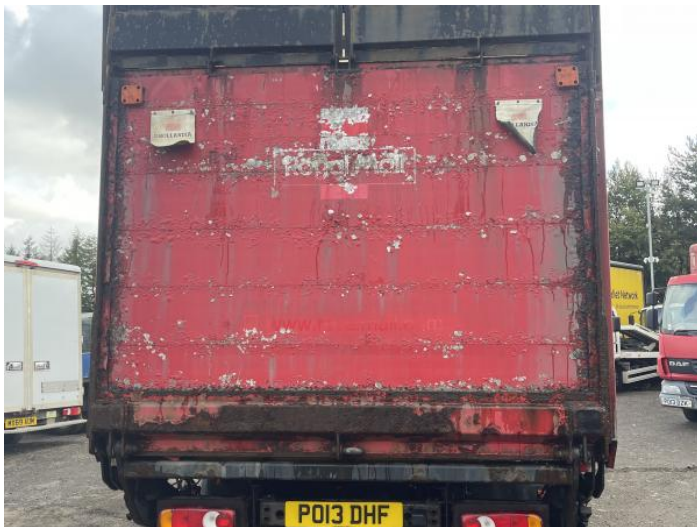
9: Tailgate Rusted Over 5mm
