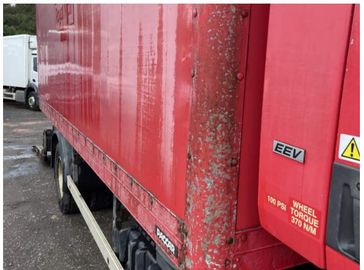
8: Qtr Panel osr Rusted Over 5mm
