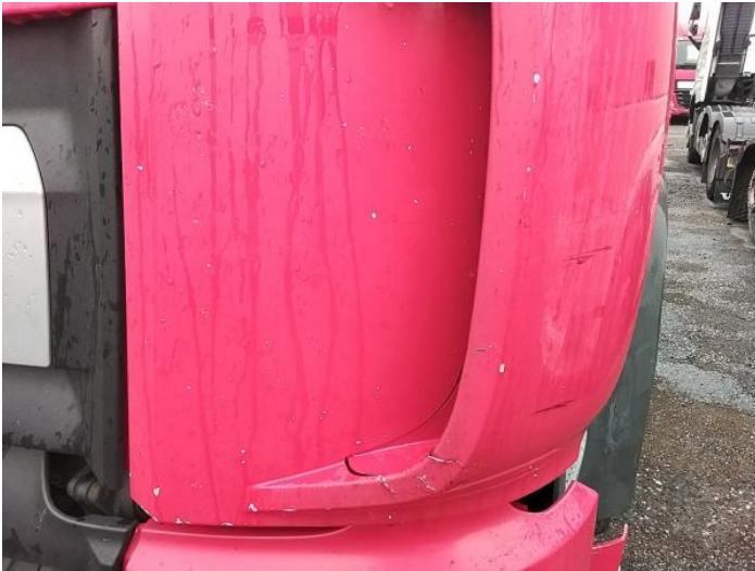
3: Panel Front Cracked Replace
