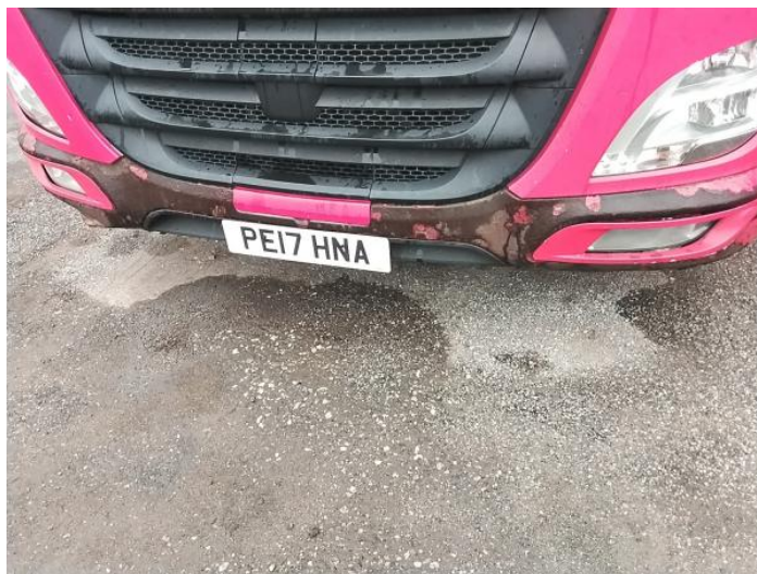
2: Bumper Front Rusted Over 5mm
