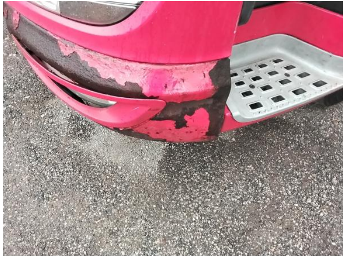
4: Bumper Front Dented With Paint Damage
