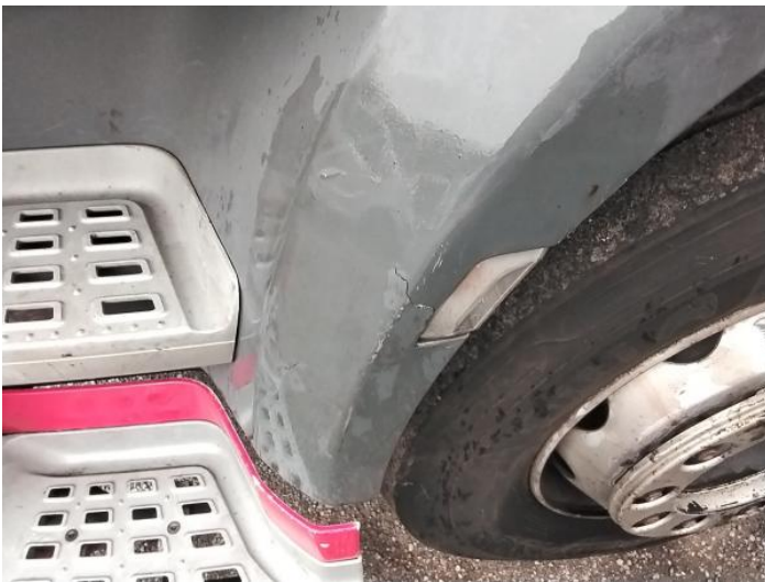
5: Wing nsf Cracked Replace
