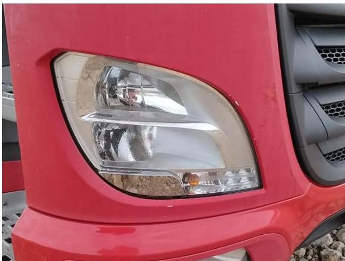
1: Fog Lamp Surround os Scratched (Painted) UpTo 25mm Thru Paint
