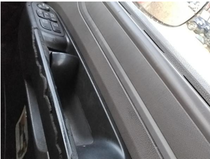
11: Door Pad osf Torn Over 10mm
