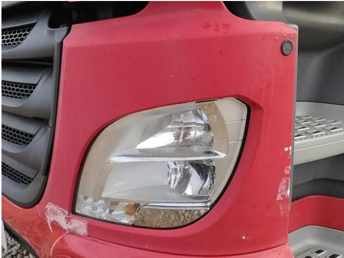
4: Fog Lamp Surround ns Broken Replace
