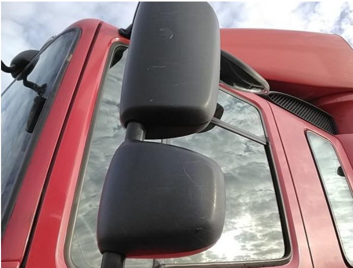
5: Door Mirror Assy nsf Scuffed (Unpainted) UpTo 100mm
