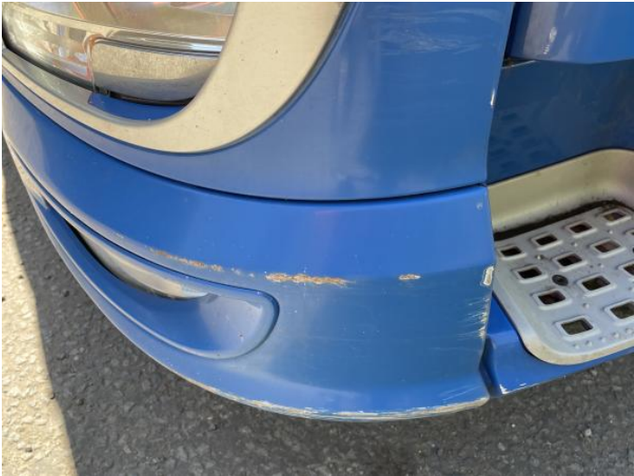
3: Bumper Front Scratched Over 100mm Thru Paint
