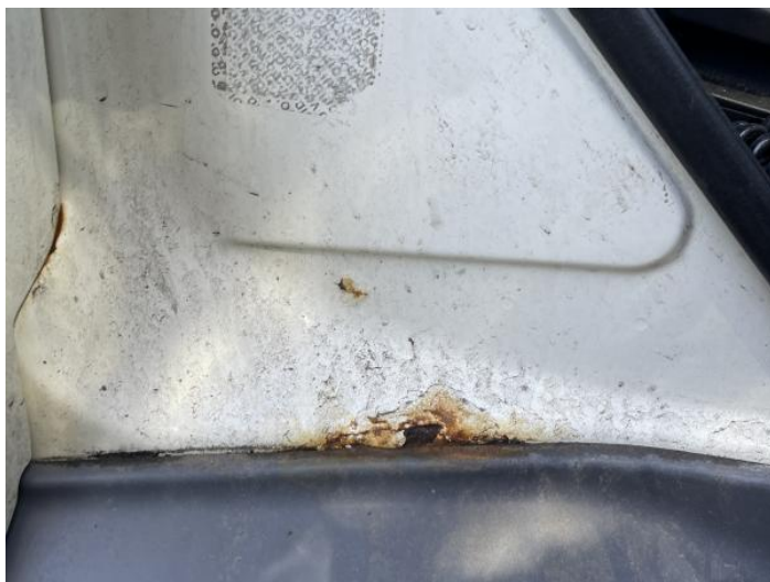
1: Sill os Rusted Over 5mm
