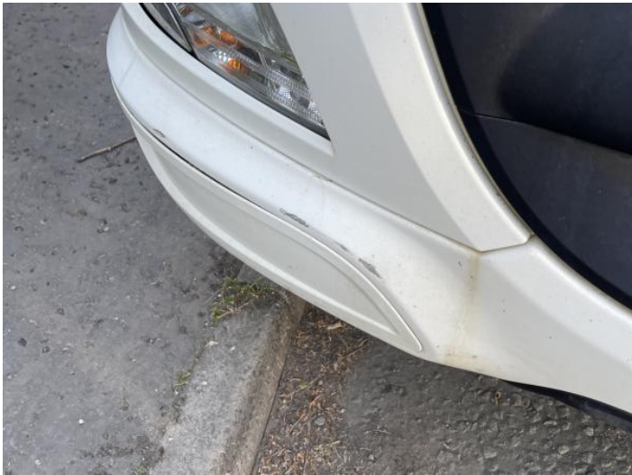
6: Bumper Front Scratched 25 to 100mm Thru Paint
