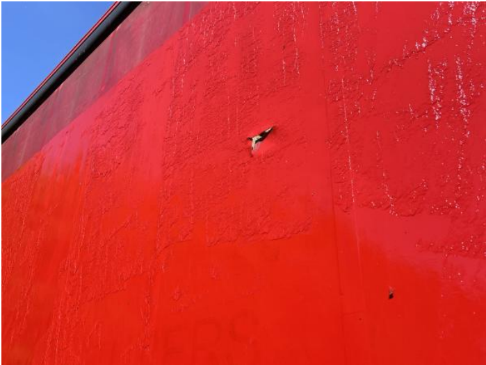
3: Qtr Panel osr Dented Over 30mm
