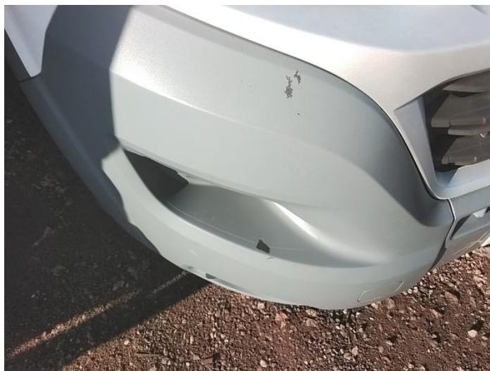
2: Bumper Front Scratched 25 to 100mm Thru Paint
