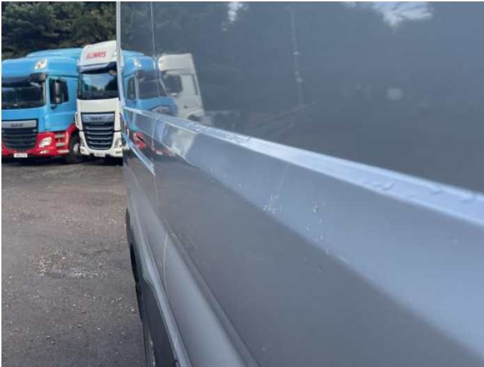
3: Qtr Panel osr Dented Over 30mm
