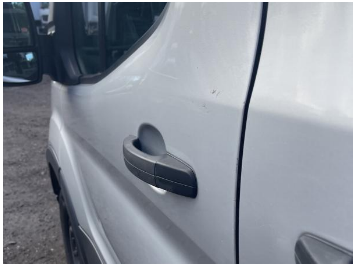
6: Door nsf Dented Over 30mm
