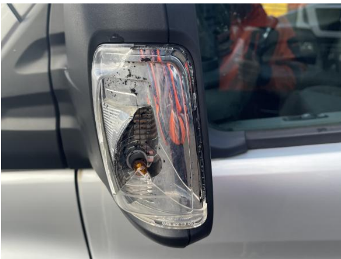
7: Flasher Side Repeater ns Broken Replace
