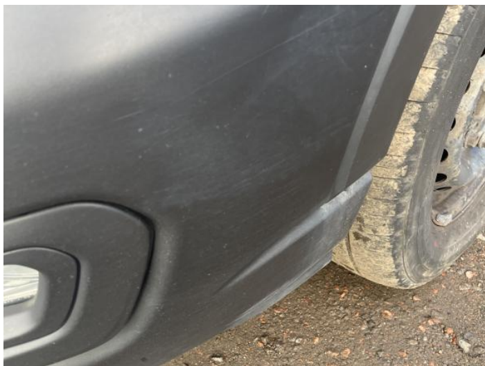
1: Bumper Front Moulding Scuffed (Unpainted) Over 100mm
