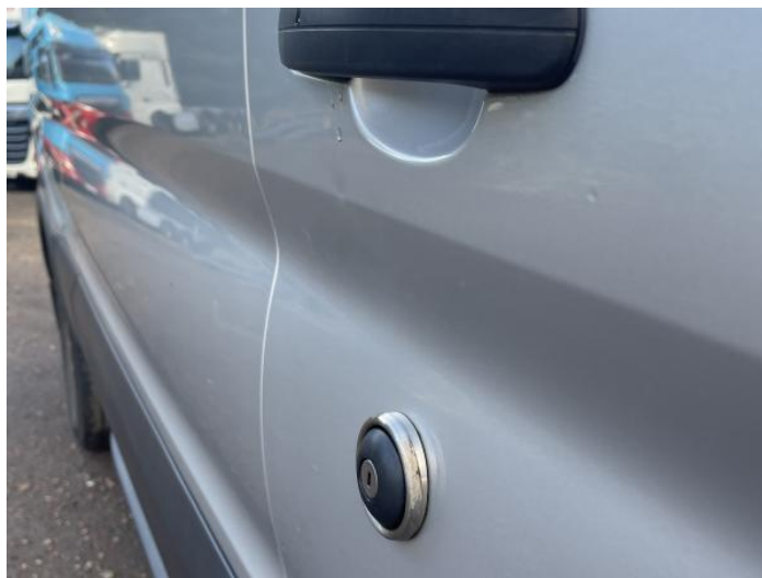
2: Door osf Dented Over 30mm
