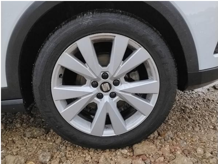
2: Wheel osf Scratched Over 50mm
