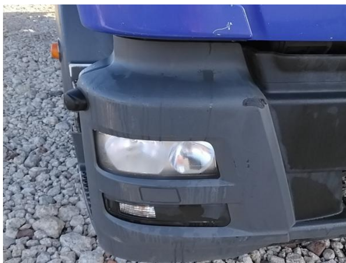
2: Fog Lamp Surround of Scuffed (Unpainted) Up To 100mm
