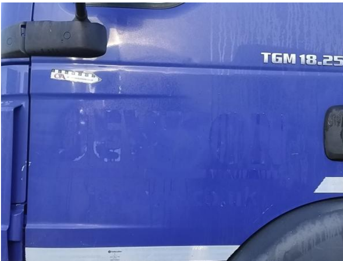
5: Door nsf Scratched Over 25mm Thru Paint
