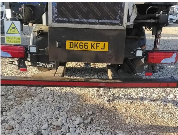
7: Bumper Rear Rusted Over 5mm
