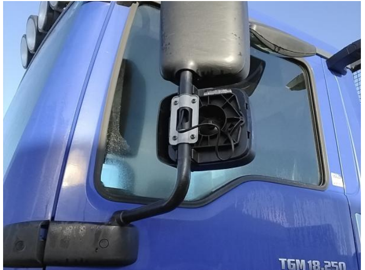
4: Door Mirror Assy nsf Missing Replace
