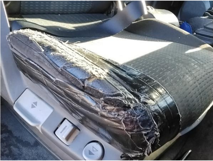
10: Seat Base Cover osf Torn Over 3mm
