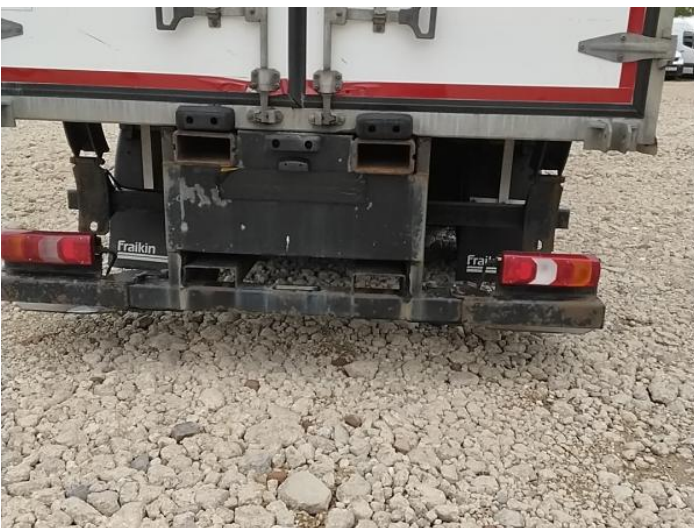
7: Bumper Rear Rusted Over 5mm
