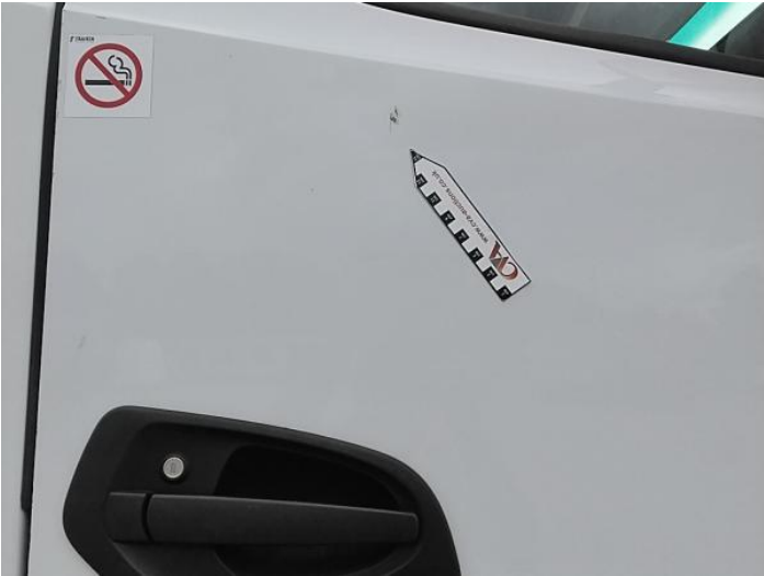
10: Door osf Scratched UpTo 25mm Thru Paint
