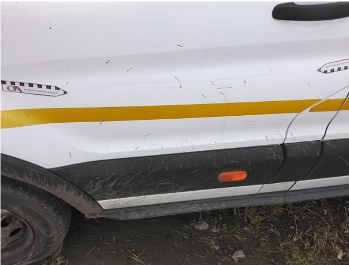
5: Door nsf Scratched Over 25mm Thru Paint
