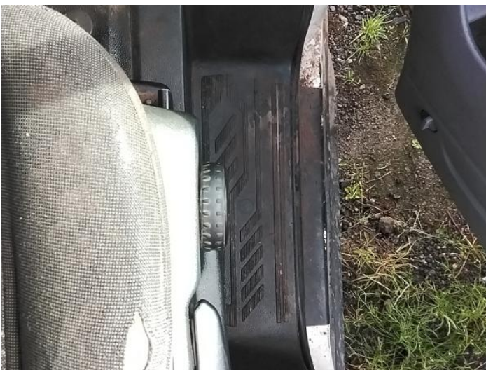
19: Seat Base Cover osf Holed Over 3mm
