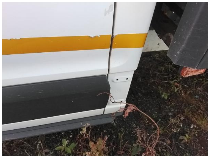
8: Door Moulding nsr Missing Replace
