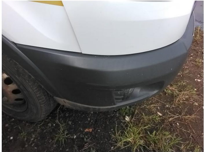
10: Bumper Front Scratched Over 100mm Thru Paint
