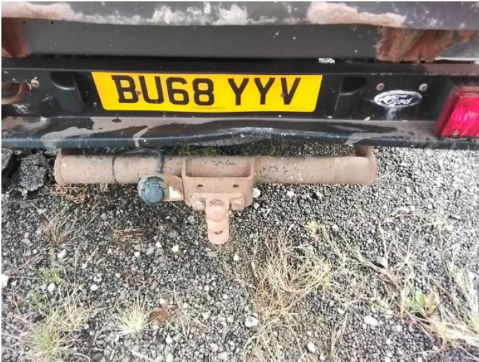
9: Bumper Rear Dented Over 30mm
