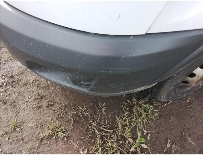
3: Bumper Front Scratched Over 100mm Thru Paint
