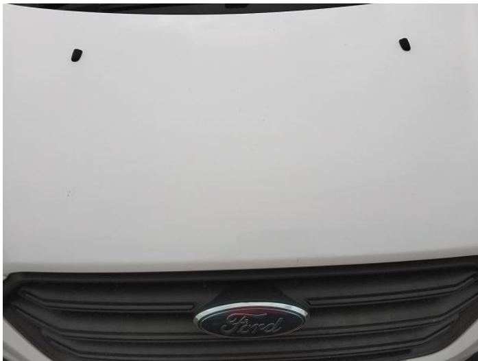
1: Bonnet Chipped Multiple Chips
