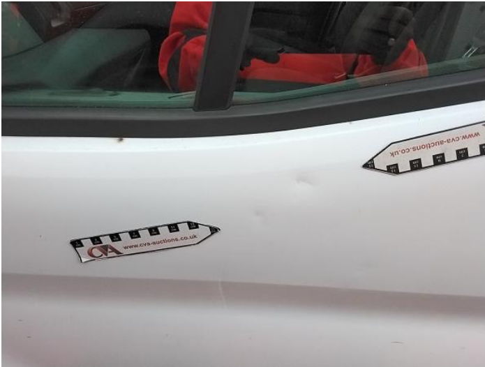
3: Door nsf Dented Over 30mm
