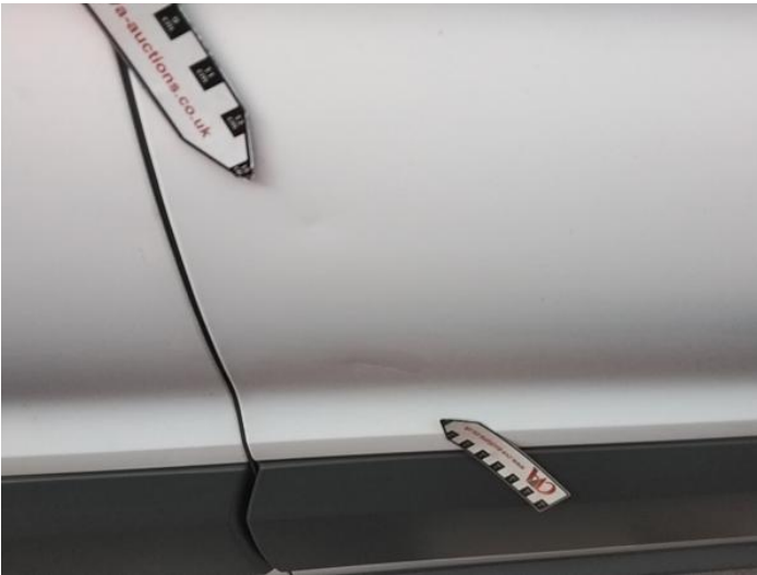
11: Qtr Panel osr Dented With Paint Damage
