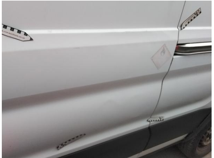
4: Qtr Panel nsr Dented Over 30mm
