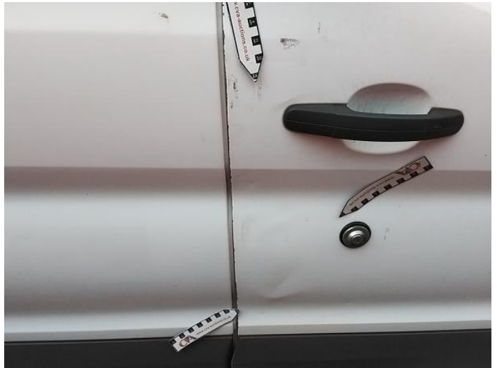
12: Door osf Dented With Paint Damage
