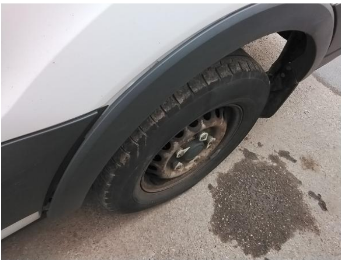
7: Qtr Panel Moulding ns Broken Replace
