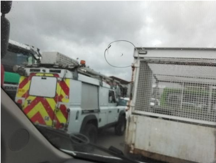
15: Screen Front Chipped Over 10mm
