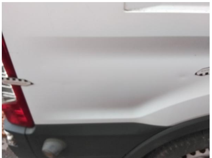
8: Qtr Panel osr Dented Over 30mm
