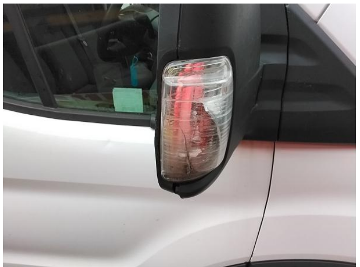
14: Door Mirror Assy osf Broken Replace
