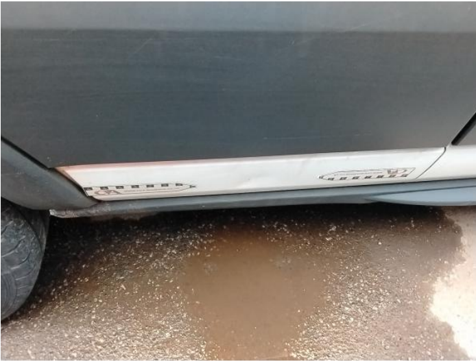
9: Qtr Panel osr Dented Over 30mm
