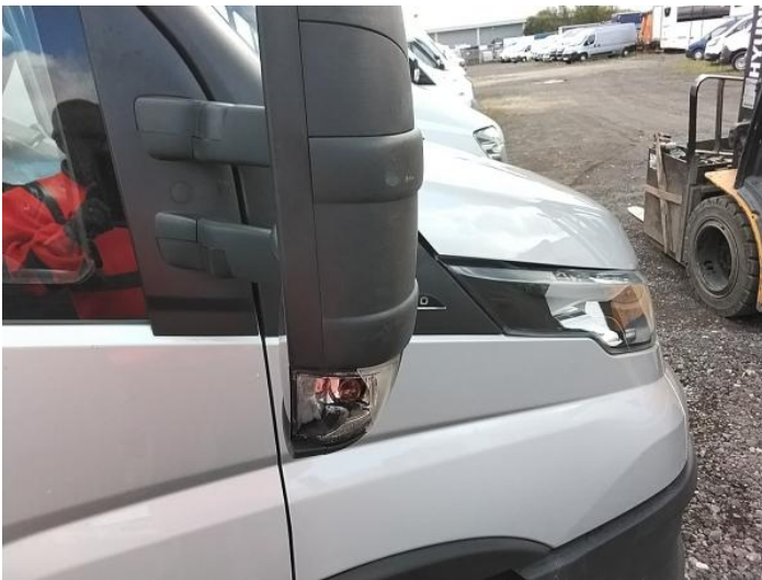
5: Door Mirror Assy osf Broken Replace
