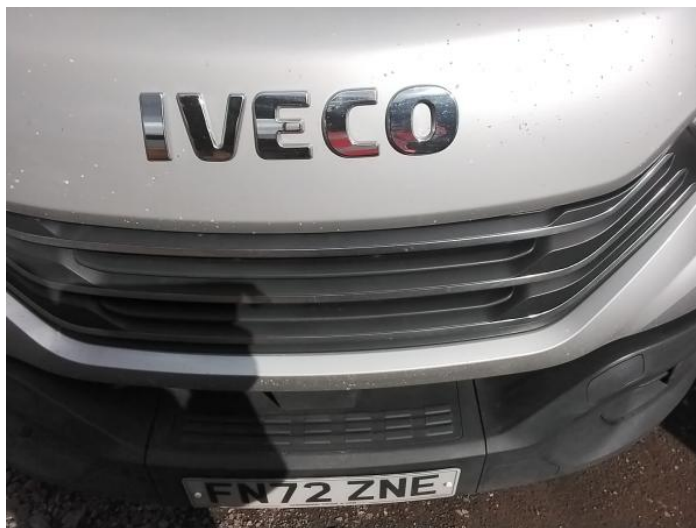
2: Panel Front Chipped Multiple Chips
