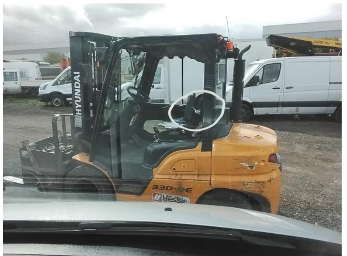
8: Screen Front Chipped Over 10mm
