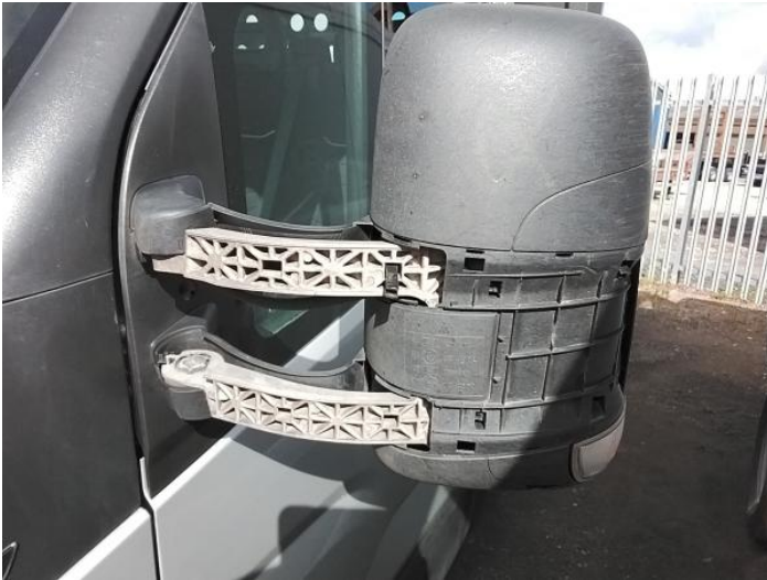
3: Door Mirror Assy nsf Broken Replace
