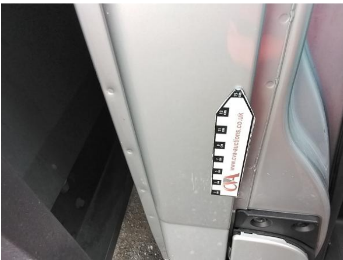
7: B Post os Scratched Over 25mm Thru Paint
