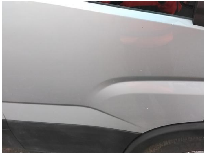
6: Door osf Chipped Multiple Chips
