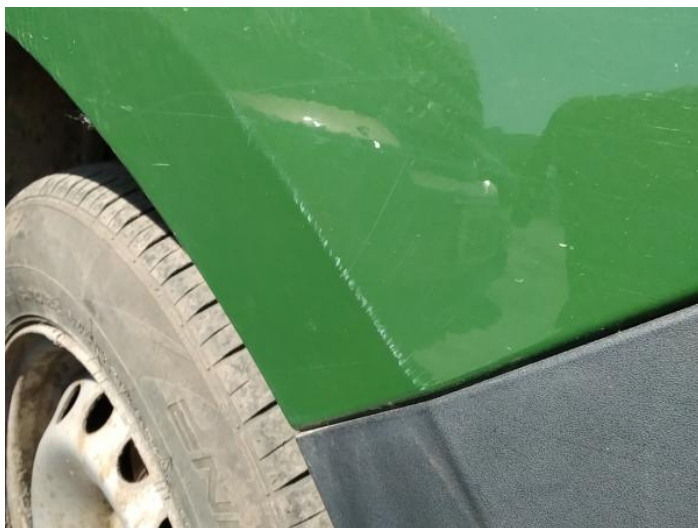
1: Moulding nsf Wing Scratched (Painted) Over 25mm Not Thru Paint
