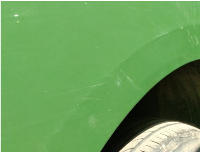
7: Panel Rear Scratched Over 25mm Not Thru Paint
