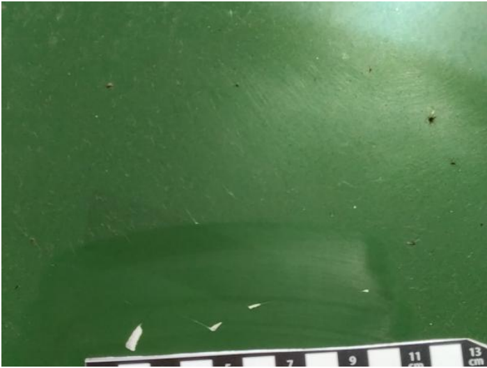
15: Bonnet Scratched UpTo 25mm Thru Paint
