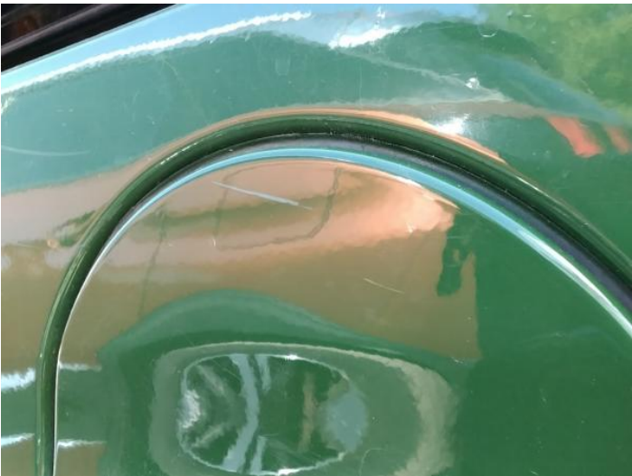
8: Fuel Flap Scratched Over 25mm Not Thru Paint
