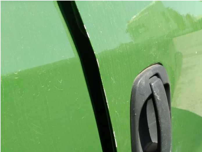
3: Door nsf Chipped Multiple Chips
