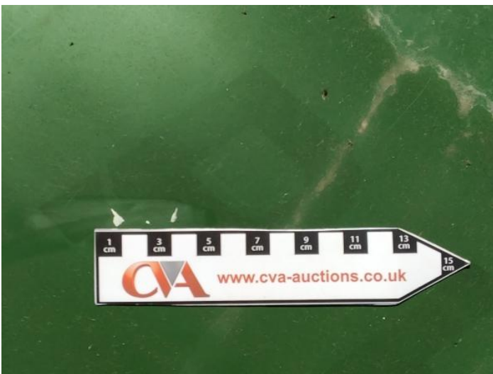
13: Bonnet Scratched UpTo 25mm Thru Paint
