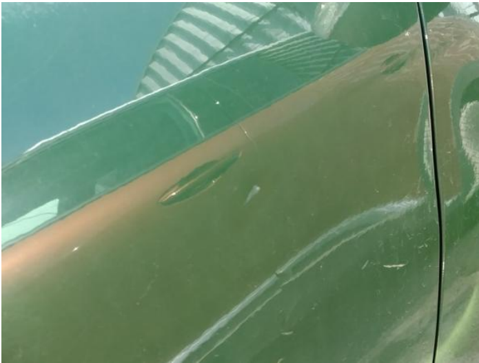
11: Wing osf Dented With Paint Damage
