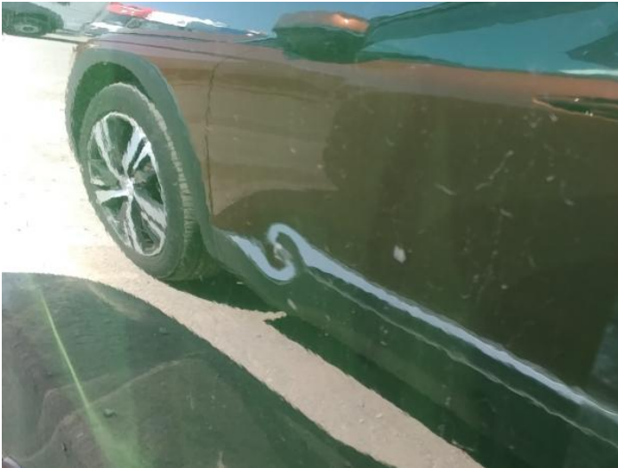
9: Door osf Dented With Paint Damage
