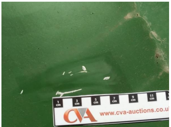
14: Bonnet Scratched Over 25mm Thru Paint
