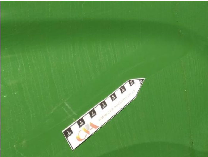
6: Panel Rear Scratched Over 25mm Not Thru Paint
