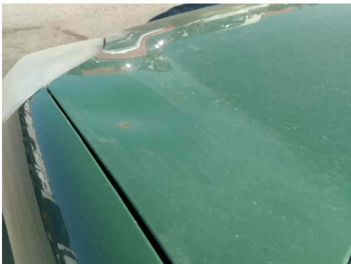
15: Bonnet Dented Over 30mm
