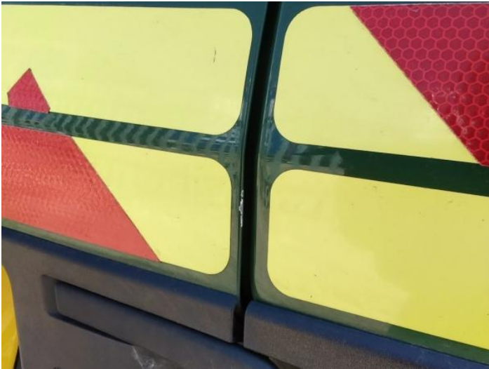
9: Panel Rear Chipped Edge Chip
