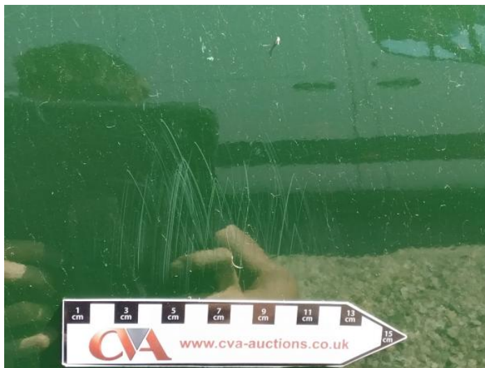
2: Door nsf Scratched Over 25mm Not Thru Paint
