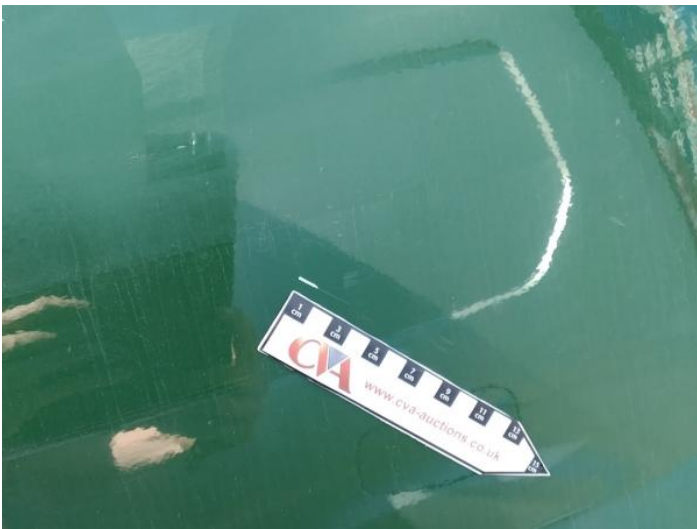
11: Panel Rear Scratched UpTo 25mm Thru Paint
