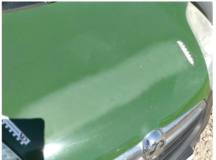
6: Bonnet Scratched Over 25mm Not Thru Paint
