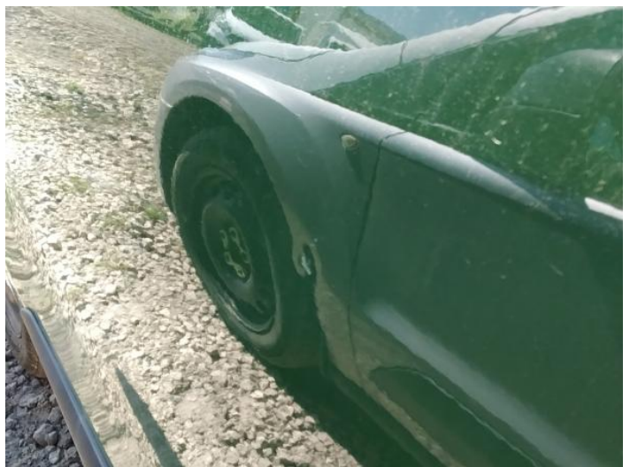
14: Door osf Dented With Paint Damage
