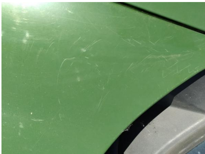
1: Bonnet Scratched UpTo 25mm Not Thru Paint
