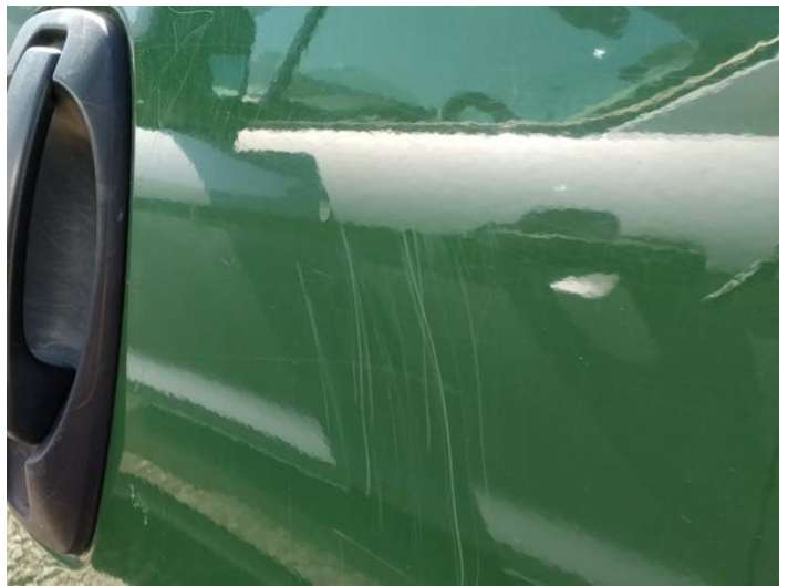
12: Panel Rear Scratched Over 25mm Not Thru Paint
