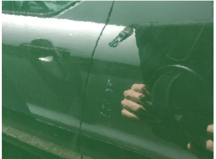
10: Panel Rear Scratched Over 25mm Not Thru Paint
