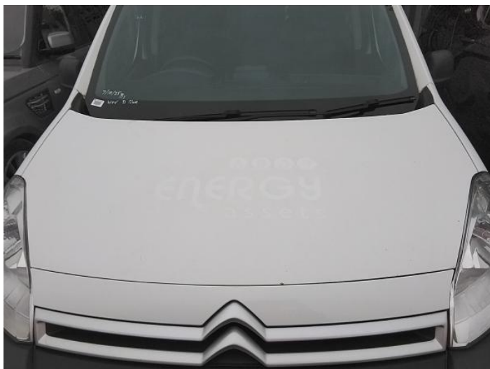
1: Bonnet Chipped Multiple Chips
