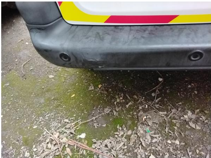
3: Bumper Rear Poor Previous Repair Rippled UpTo 30%
