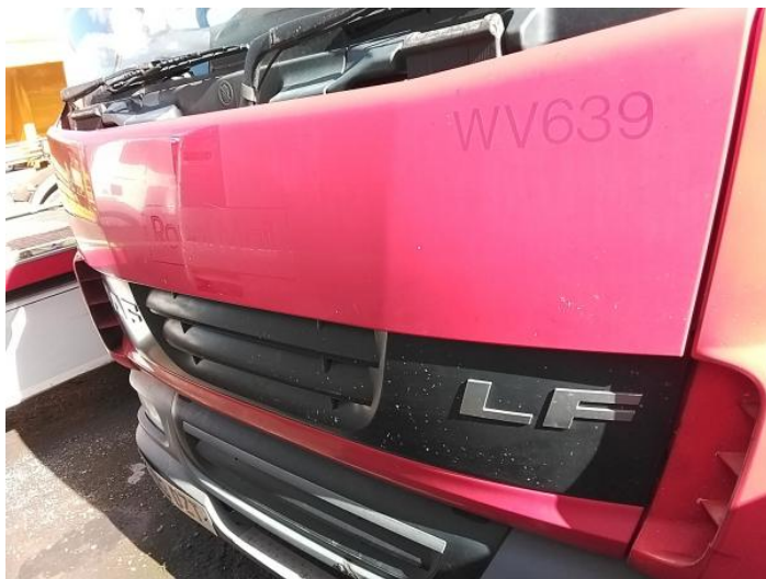
1: Bonnet Chipped Multiple Chips
