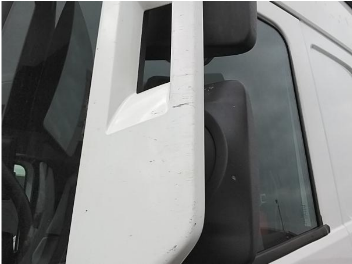
4: Door Mirror Assy osf Scuffed (Unpainted) Over 100mm
