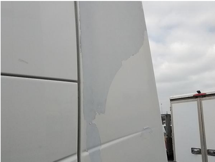
5: Panel Front Scratched Over 25mm Thru Paint
