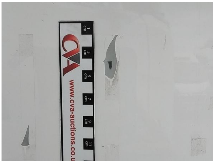
1: Door nsf Scratched Over 25mm Thru Paint
