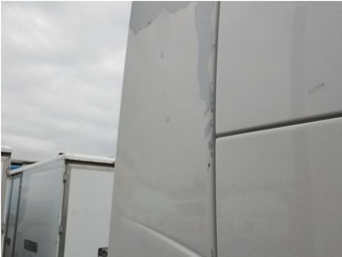
3: Panel Front Scratched Over 25mm Thru Paint
