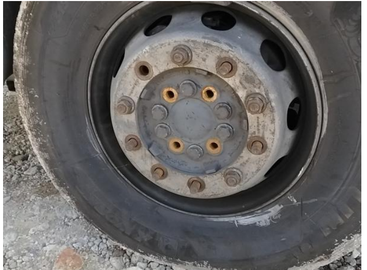
10: Wheel nsf Missing Replace
