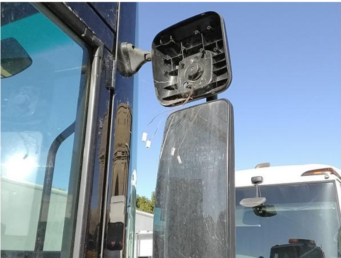
25: Door Mirror Glass os Missing Replace
