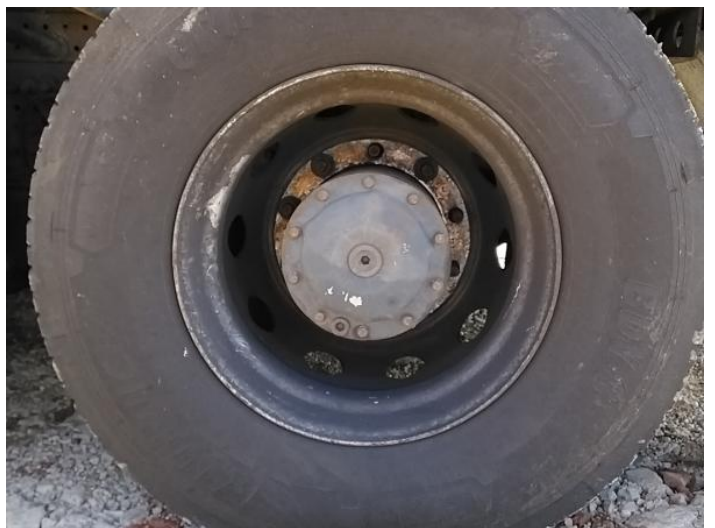
14: Wheel nsr Missing Replace
