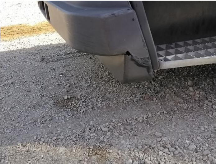
3: Bumper Front Cracked Over 25mm
