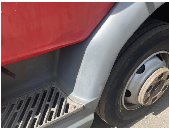
12: Door Moulding nsf Scuffed (Unpainted) Over 100mm
