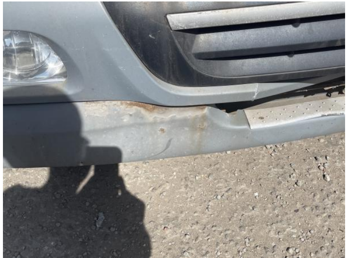
6: Bumper Front Rusted Over 5mm
