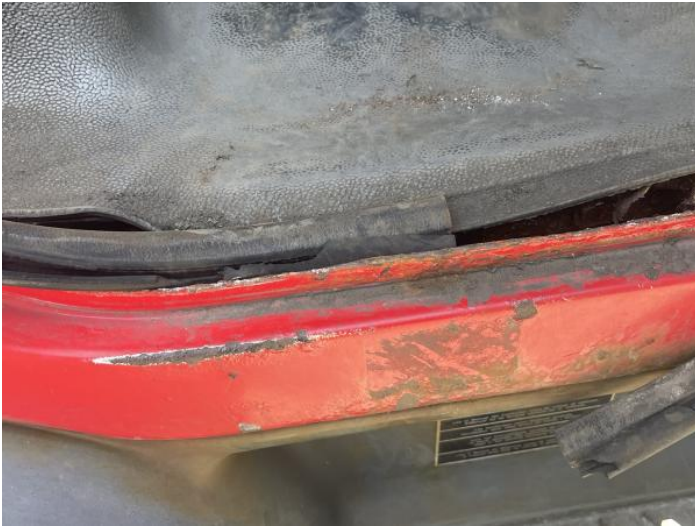
3: Sill os Rusted Over 5mm
