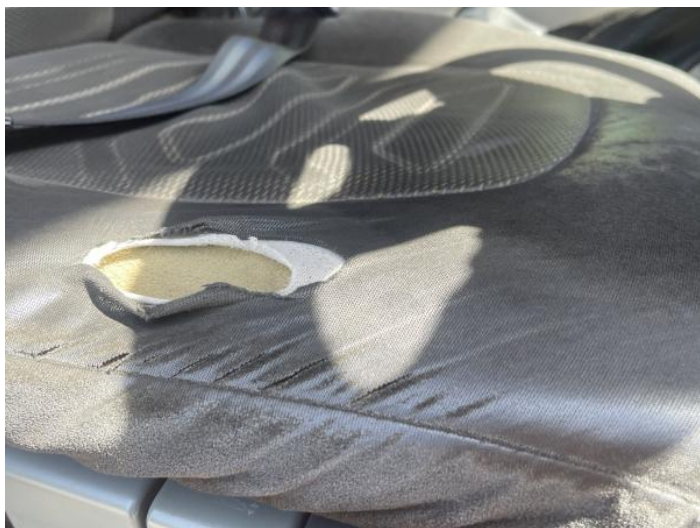
1: Seat Base Cover osf Torn Over 3mm
