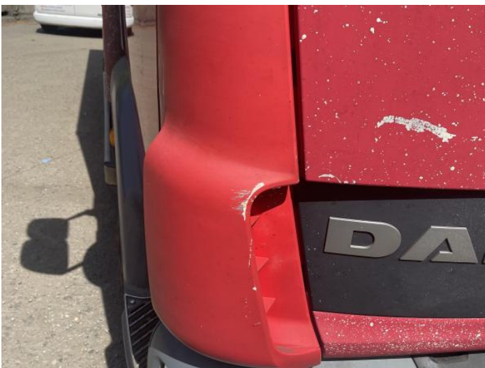
7: Wing osf Scratched Over 25mm Thru Paint
