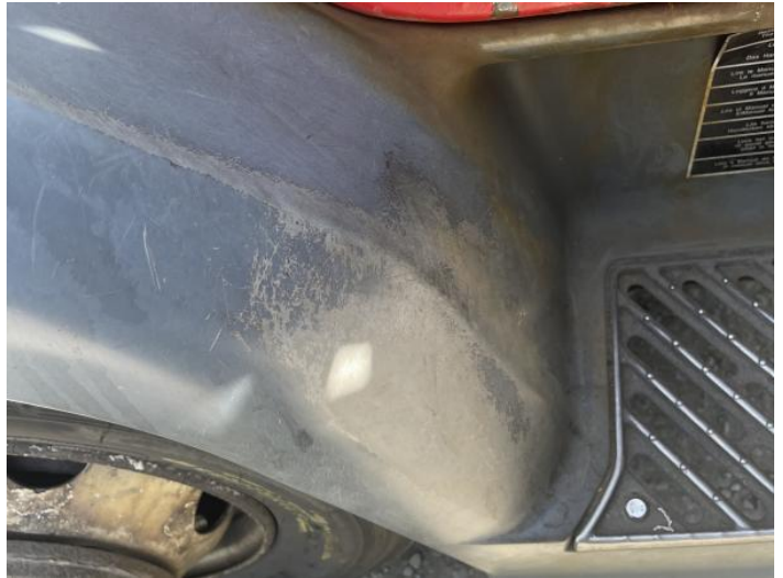
4: Door Moulding osf Scuffed (Unpainted) Over 100mm
