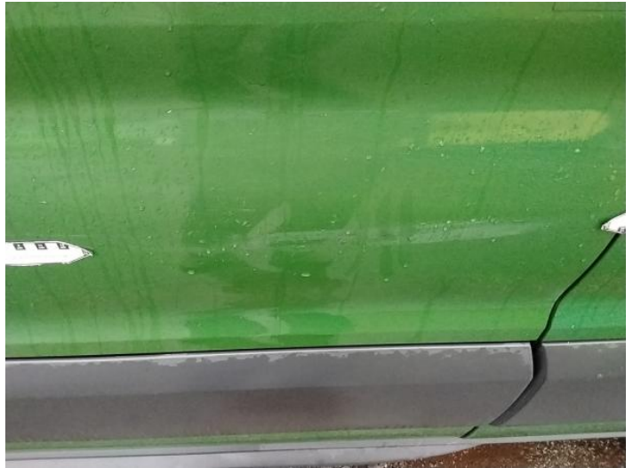
4: Qtr Panel nsr Scratched Over 25mm Thru Paint
