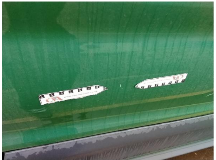
6: Qtr Panel osr Dented With Paint Damage
