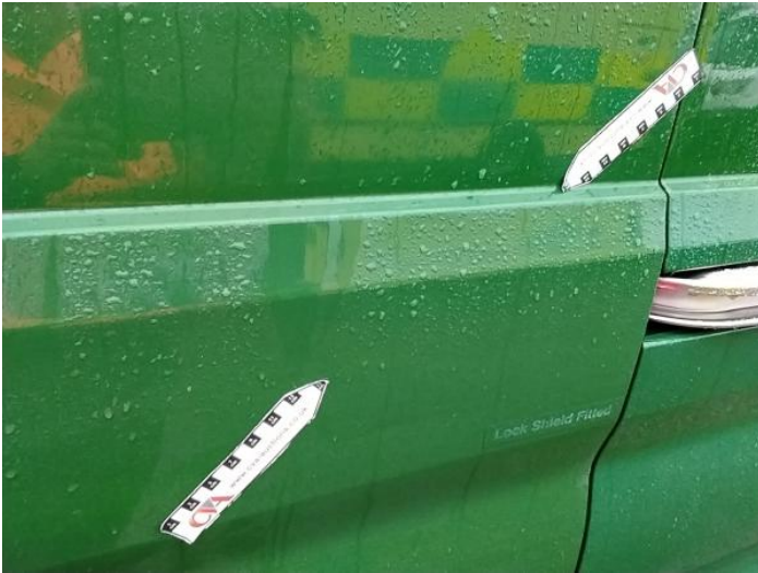
3: Qtr Panel nsr Dented Over 30mm
