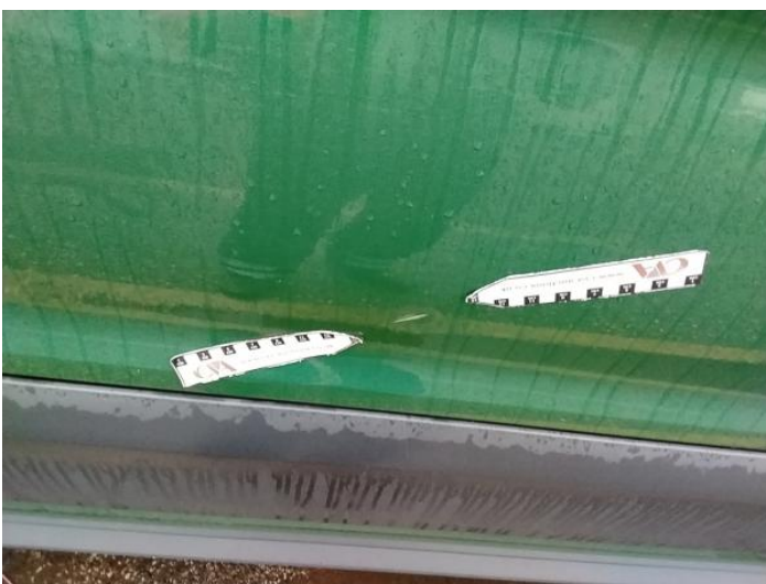
7: Qtr Panel osr Dented With Paint Damage
