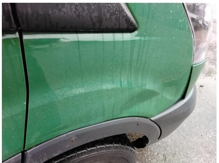
8: Wing osf Dented Over 30% Of Panel
