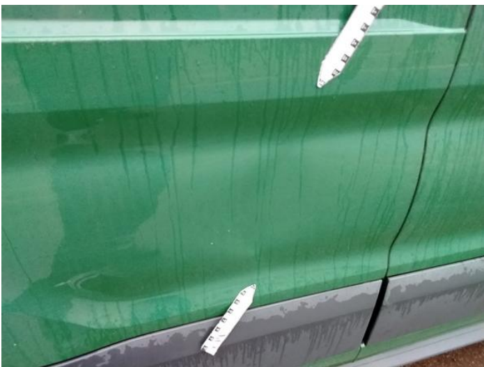
13: Qtr Panel osr Dented Over 30mm
