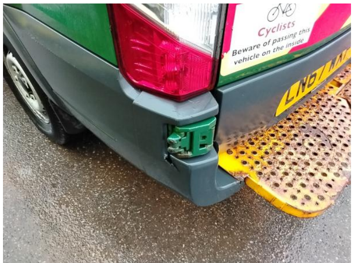
8: Bumper Rear Moulding Broken Replace
