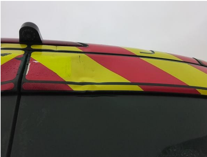
11: Door osr Dented With Paint Damage
