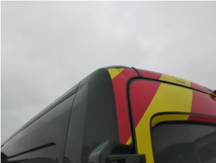
9: C Post ns Dented With Paint Damage
