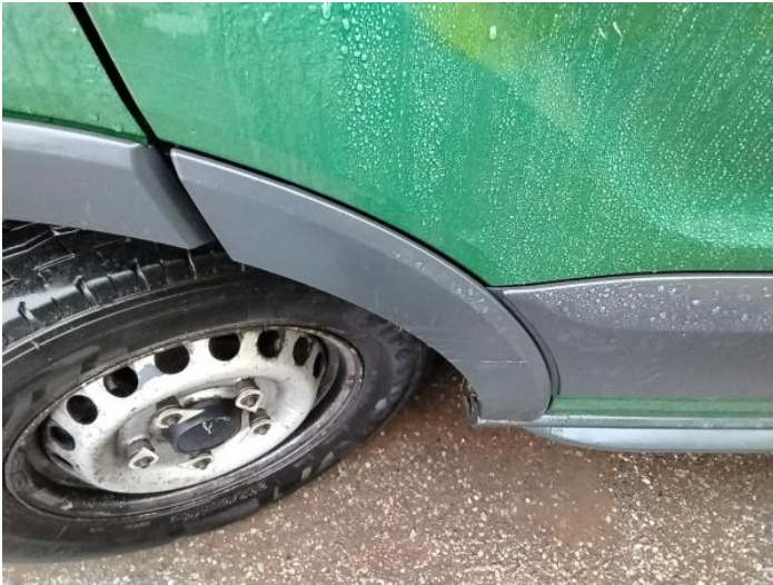
3: Door Moulding nsf Scuffed (Unpainted) UpTo 100mm
