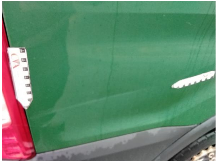
12: Qtr Panel osr Dented With Paint Damage
