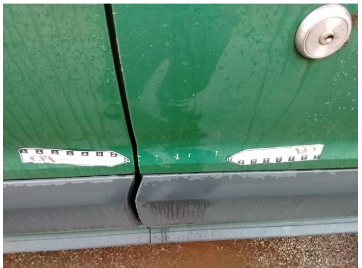
14: Door osf Scratched Over 25mm Thru Paint
