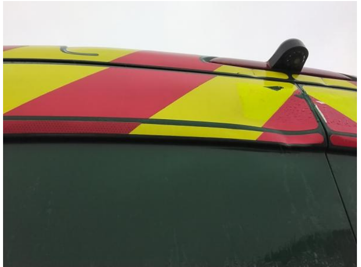
10: Door nsr Dented With Paint Damage
