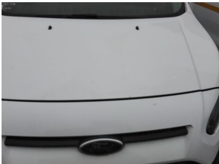
1: Bonnet Chipped Multiple Chips
