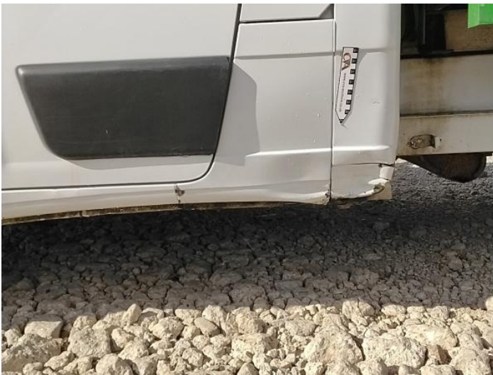
11: Sill ns Dented With Paint Damage
