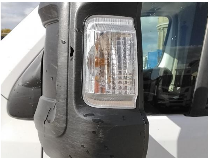
7: Flasher Side Repeater ns Broken Replace
