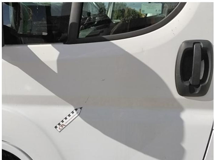
8: Door nsf Scratched UpTo 25mm Thru Paint
