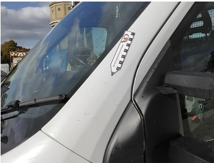
5: A Post ns Scratched Over 25mm Thru Paint
