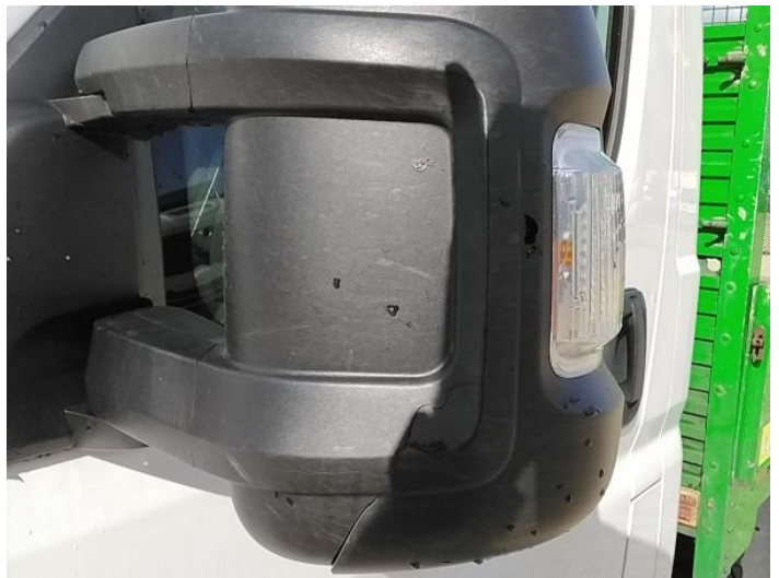
6: Door Mirror Assy nsf Broken Replace
