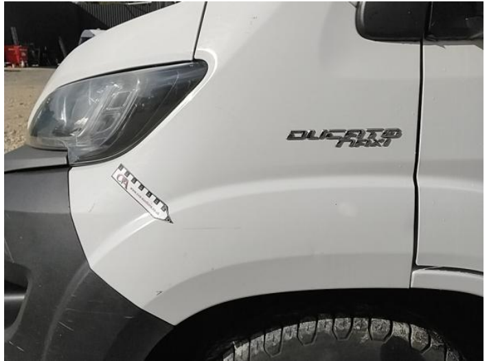
4: Wing nsf Scratched Over 25mm Thru Paint
