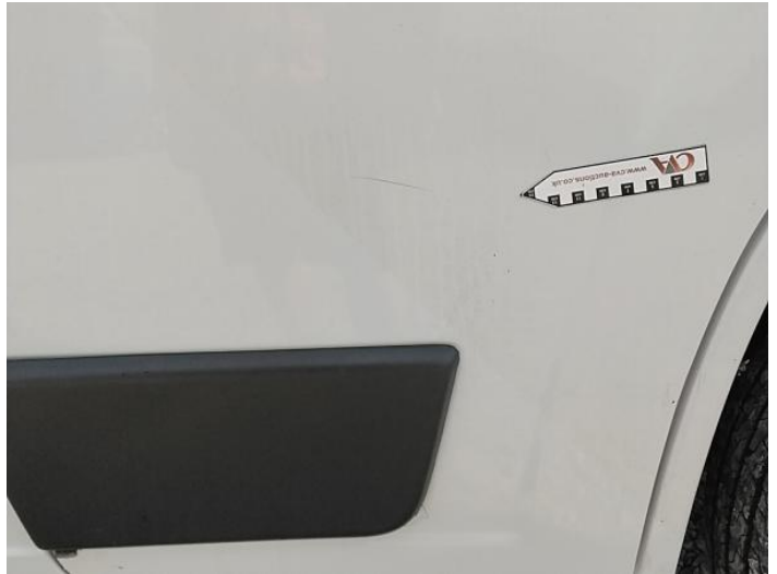
16: Door osf Dented 2 Or Less UpTo 10mm
