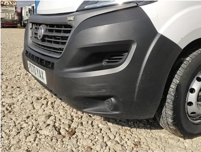
3: Bumper Front Moulding Scuffed (Unpainted) UpTo 100mm
