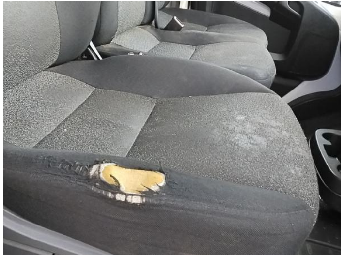
18: Seat Base Cover osf Holed Over 3mm
