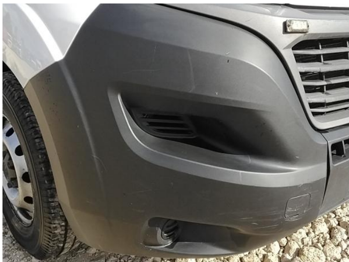
1: Bumper Front Moulding Scuffed (Unpainted) UpTo 100mm
