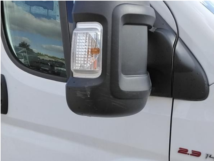
15: Door Mirror Assy osf Scuffed (Unpainted) UpTo 100mm
