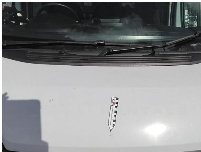
2: Bonnet Dented With Paint Damage
