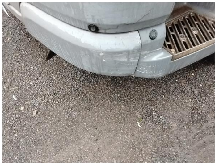
2: Bumper Front Scratched Over 100mm Thru Paint
