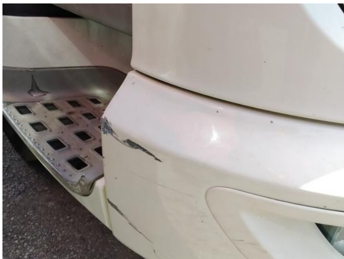
1: Bumper Front Scratched Over 100mm Thru Paint
