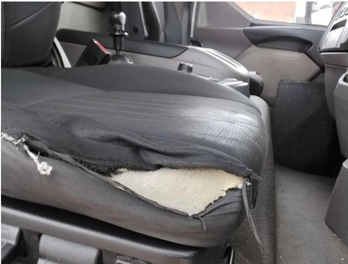
17: Seat Base Cover osf Holed Over 3mm
