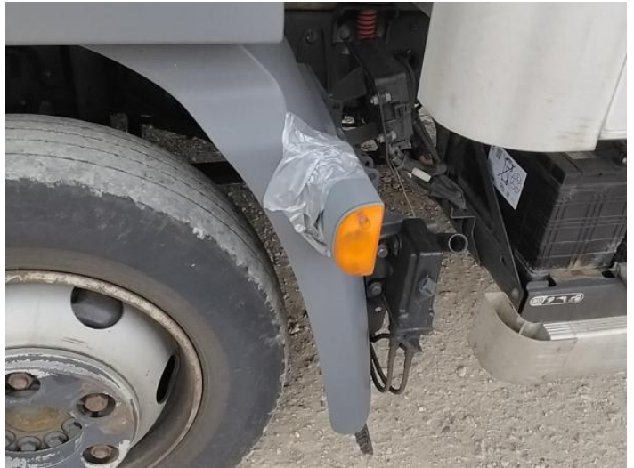
10: Flasher Side Repeater ns Broken Replace
