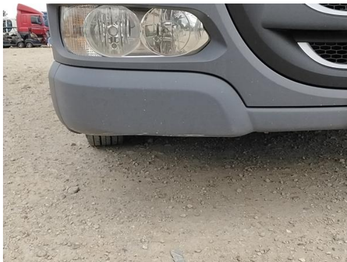
2: Bumper Front Moulding Scuffed (Unpainted) Up To 100mm
