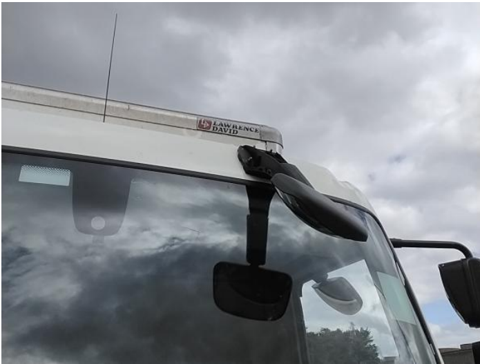
5: Door Mirror Assy nsf Missing Replace
