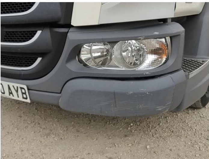
7: Fog Lamp Surround nsf Scuffed (Unpainted) UpTo 100mm
