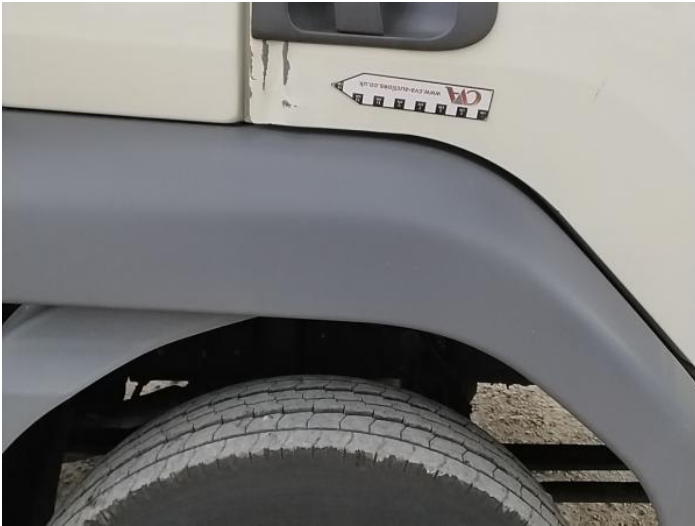
15: Door osf Dented With Paint Damage
