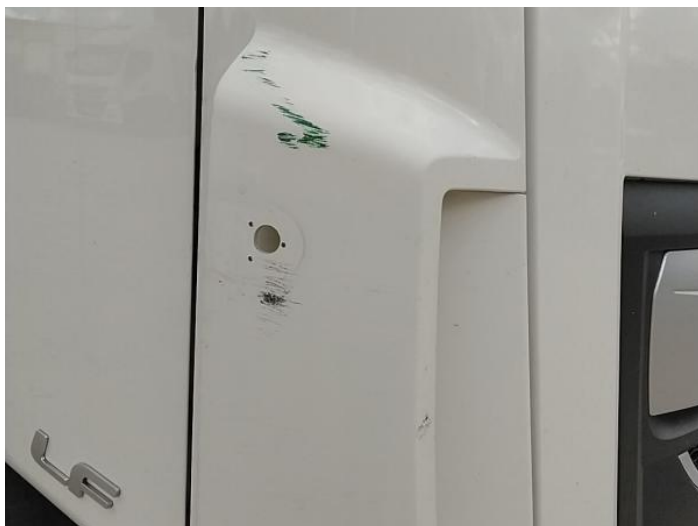
1: Wing of Scratched Over 25mm Not Thru Paint
