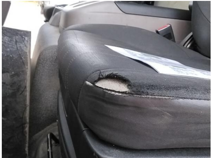
18: Seat Base Cover nsf Holed Over 3mm
