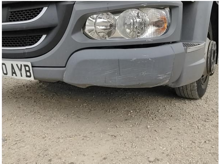
6: Bumper Front Moulding Scuffed (Unpainted) UpTo 100mm
