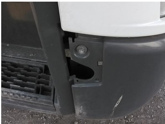
1: Bumper Front Missing Replace
