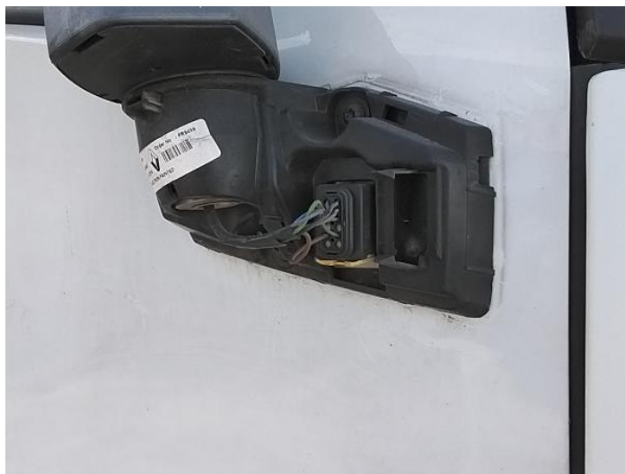
2: Door Mirror Assy nsf Broken Replace
