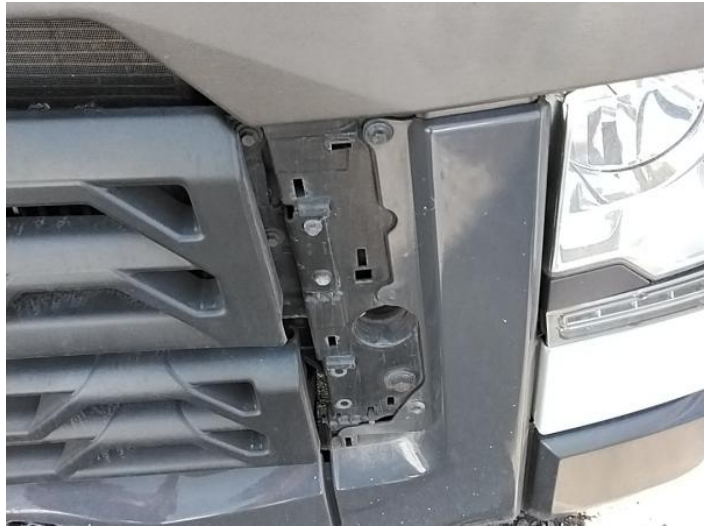
4: Bumper Front Grill Missing Replace
