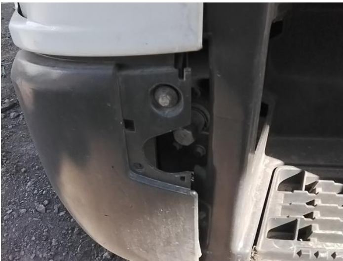
5: Bumper Front Missing Replace
