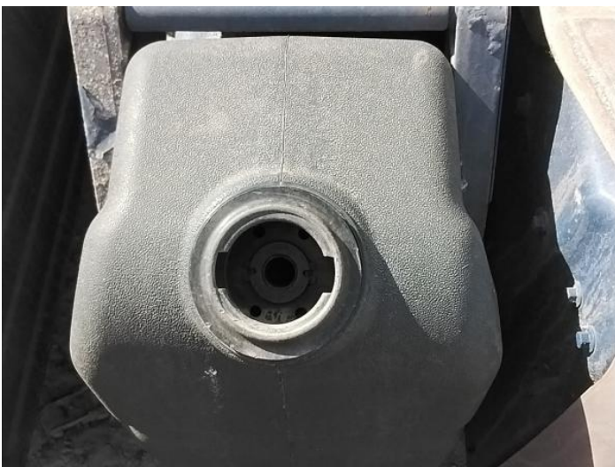
7: Fuel Flap Missing Replace
