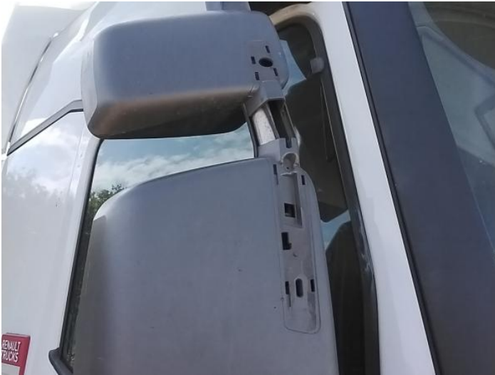
3: Door Mirror Assy nsf Broken Replace
