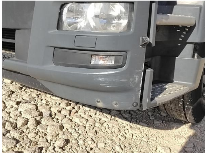
4: Fog Lamp Surround ns Scuffed (Unpainted) UpTo 100mm
