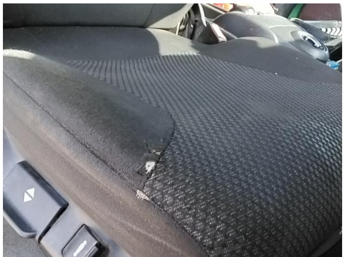
14: Seat Base Cover osf Holed Over 3mm
