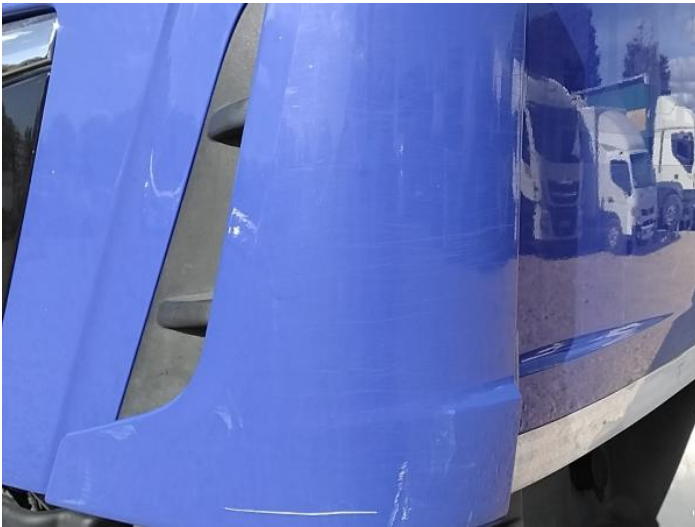
5: Wing nsf Scratched UpTo 25mm Thru Paint
