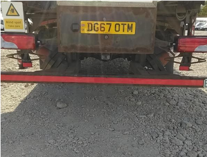
9: Bumper Rear Rusted Over 5mm
