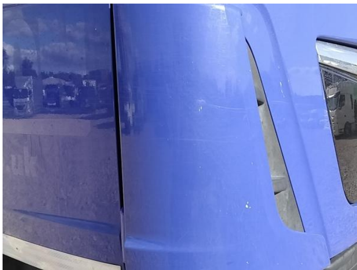
1: Wing osf Chipped Multiple Chips
