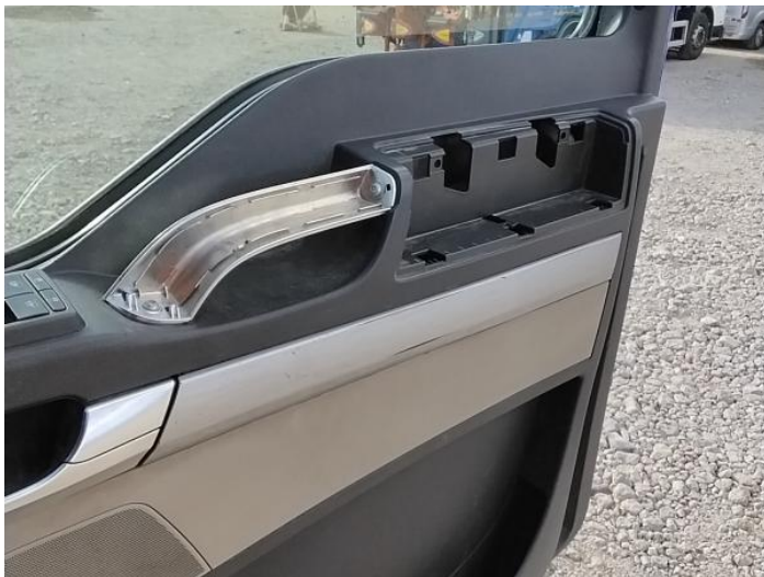
15: Handle Inner osf Damaged Replace
