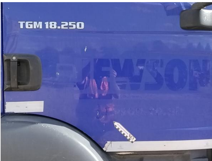
13: Door osf Scratched UpTo 25mm Thru Paint
