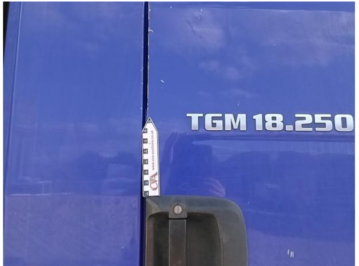
12: Door osf Chipped Edge Chip
