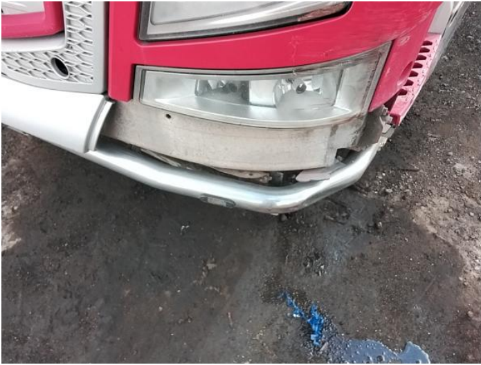
15: Bumper Front Moulding Missing Replace
