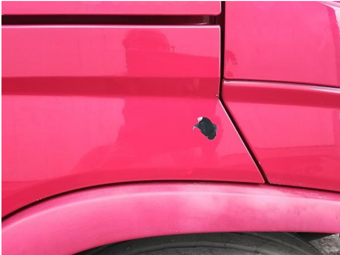
22: Qtr Panel Moulding os Scratched (Painted) Over 25mm Thru Paint
