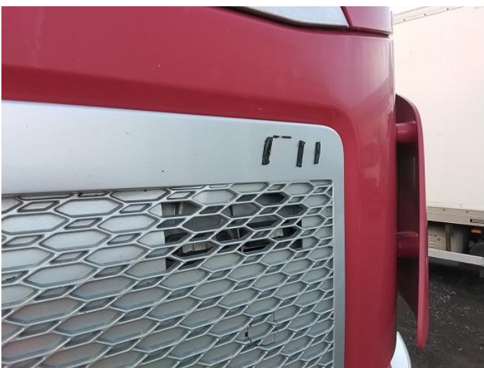
7: Badgedecal Front Missing Replace
