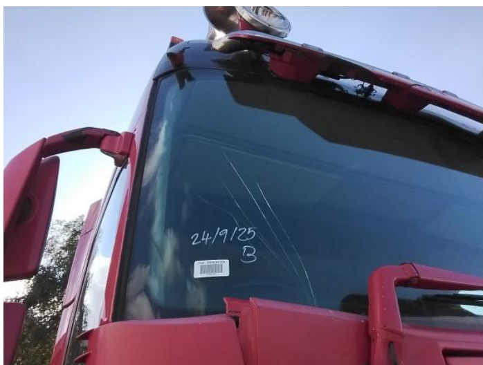
1: Screen Front Cracked Replace
