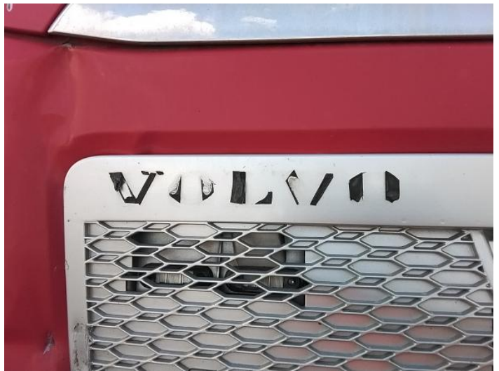
6: Badgedecal Front Missing Replace
