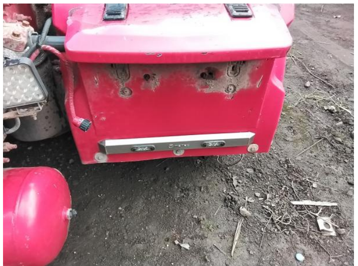
20: Lamp osr Missing Replace
