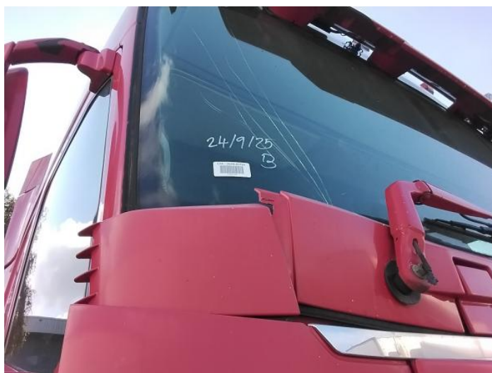
2: Panel Front Cracked Replace
