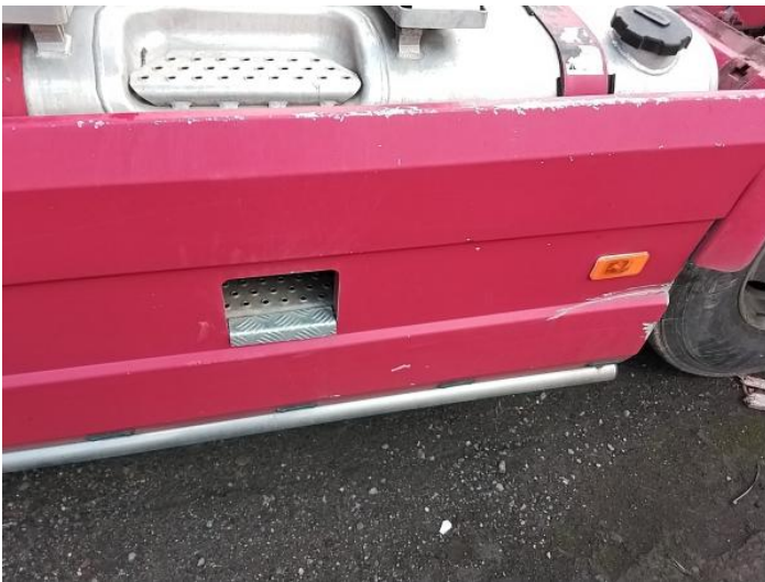
17: Qtr Panel Moulding ns Scratched (Painted) Over 25mm Thru Paint
