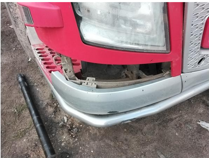
13: Bumper Front Moulding Missing Replace
