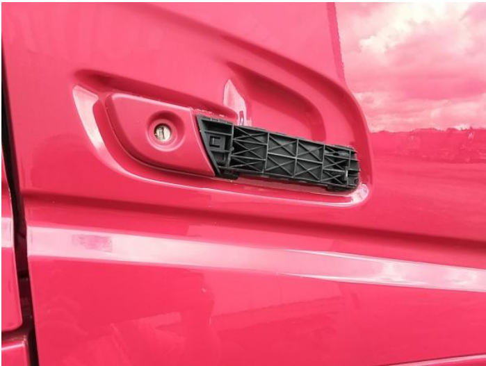
23: Door Moulding osf Missing Replace
