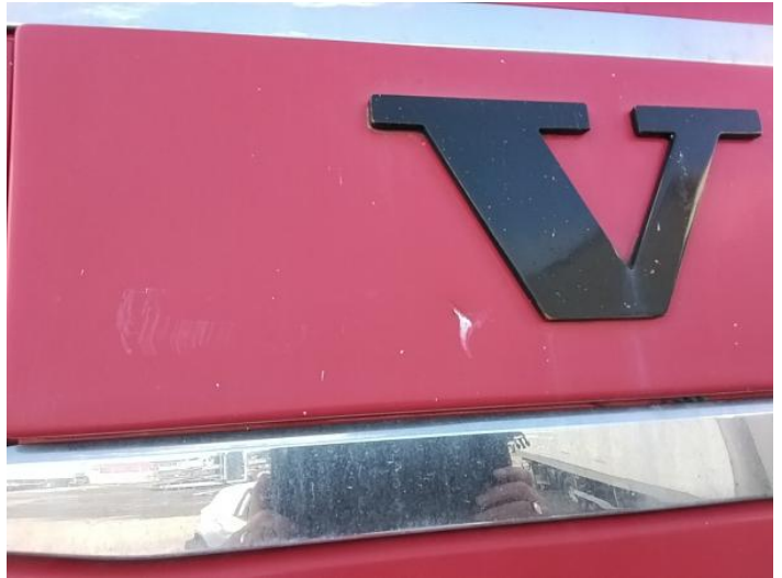
4: Panel Front Dented With Paint Damage
