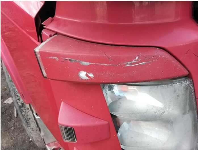
11: Panel Front Cracked Replace
