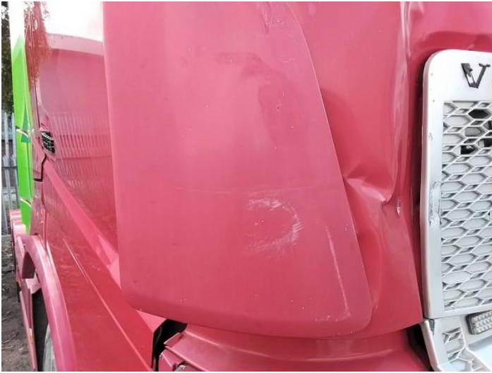
9: Panel Front Scratched Over 25mm Thru Paint
