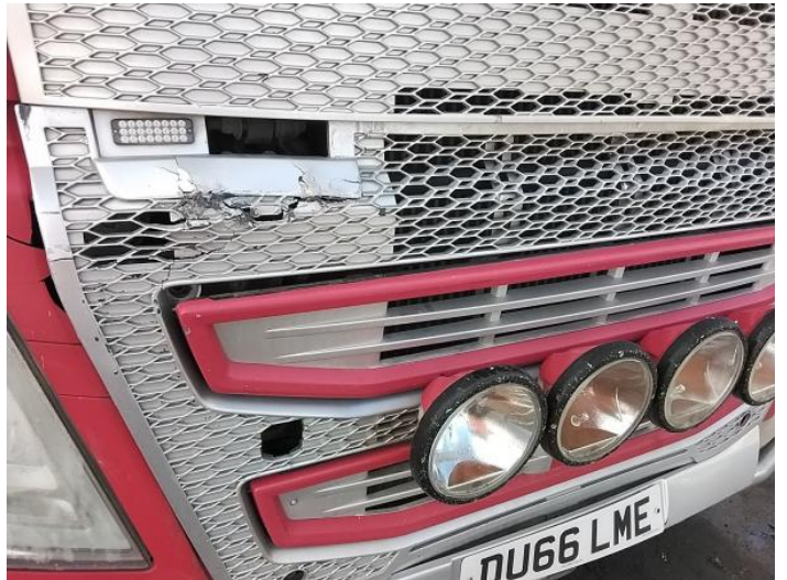
12: Bumper Front Grill Broken Replace
