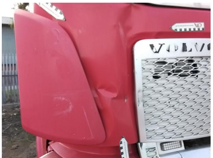
8: Bonnet Dented With Paint Damage
