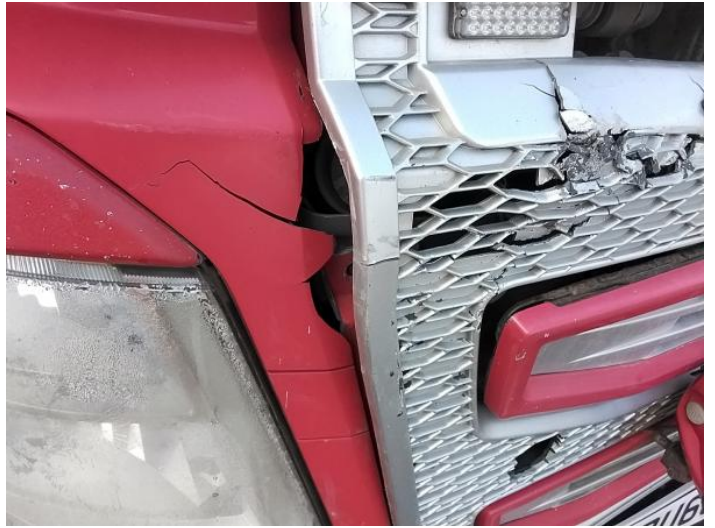
10: Panel Front Cracked Replace
