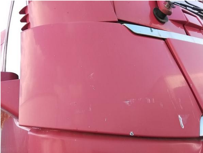
3: Panel Front Dented With Paint Damage
