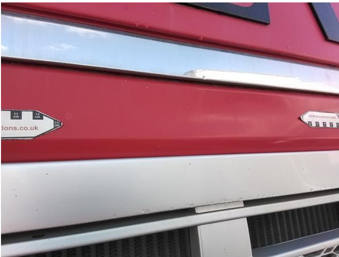
5: Bonnet Dented Over 30mm
