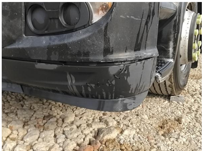
2: Bumper Front Moulding Broken Replace
