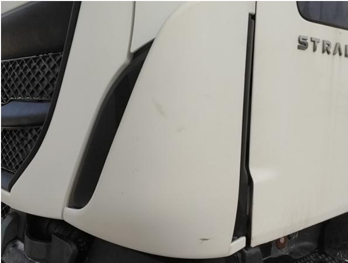
3: Wing nsf Scratched UpTo 25mm Thru Paint
