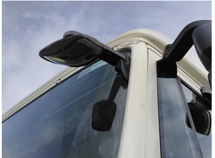
4: Door Mirror Assy nsf Broken Replace
