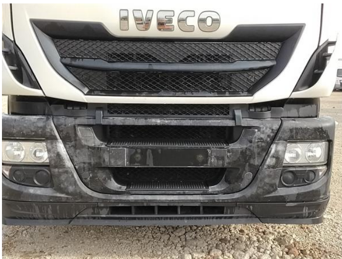
1: Bumper Front Poor Previous Repair Poor Colour
