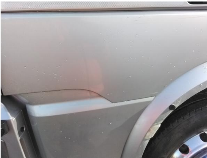
5: Door Moulding nsf Scratched (Painted) Over 25mm Thru Paint
