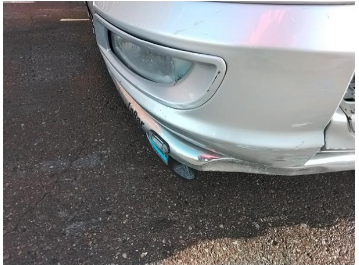
4: Bumper Front Scratched Over 100mm Thru Paint
