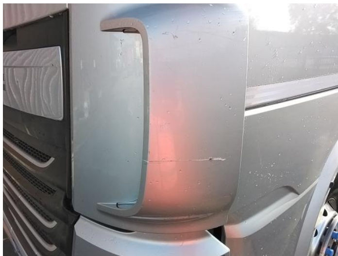
2: Panel Front Cracked Replace
