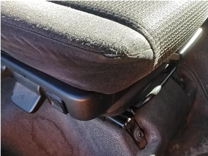
9: Seat Base Cover osf Torn Over 3mm
