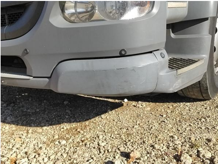
5: Bumper Front Scratched 25 to 100mm Thru Paint
