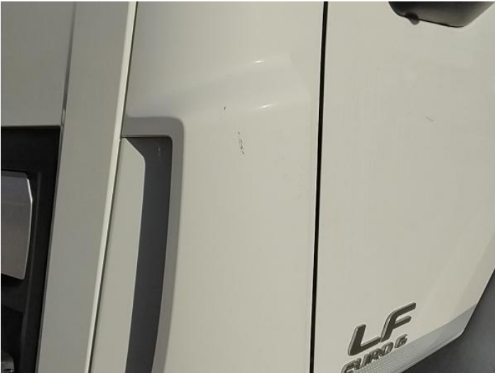
4: Wing nsf Scratched UpTo 25mm Thru Paint
