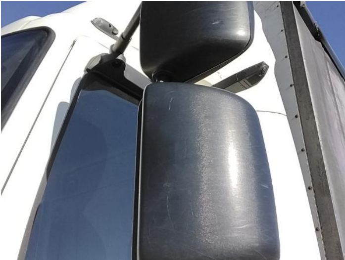
3: Door Mirror Assy nsf Scuffed (Unpainted) UpTo 100mm
