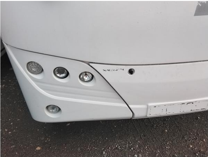
1: Panel Front Chipped Multiple Chips
