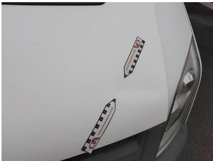
1: Bonnet Dented Over 30mm
