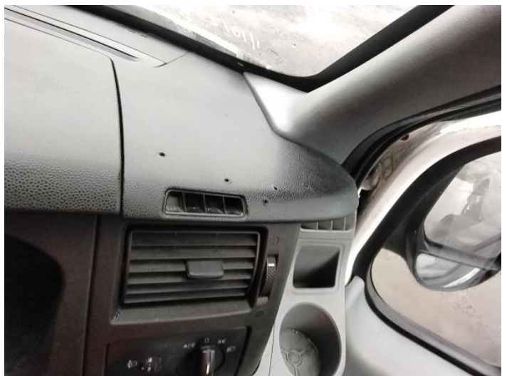
8: Fascia Panel Holed Over 3mm
